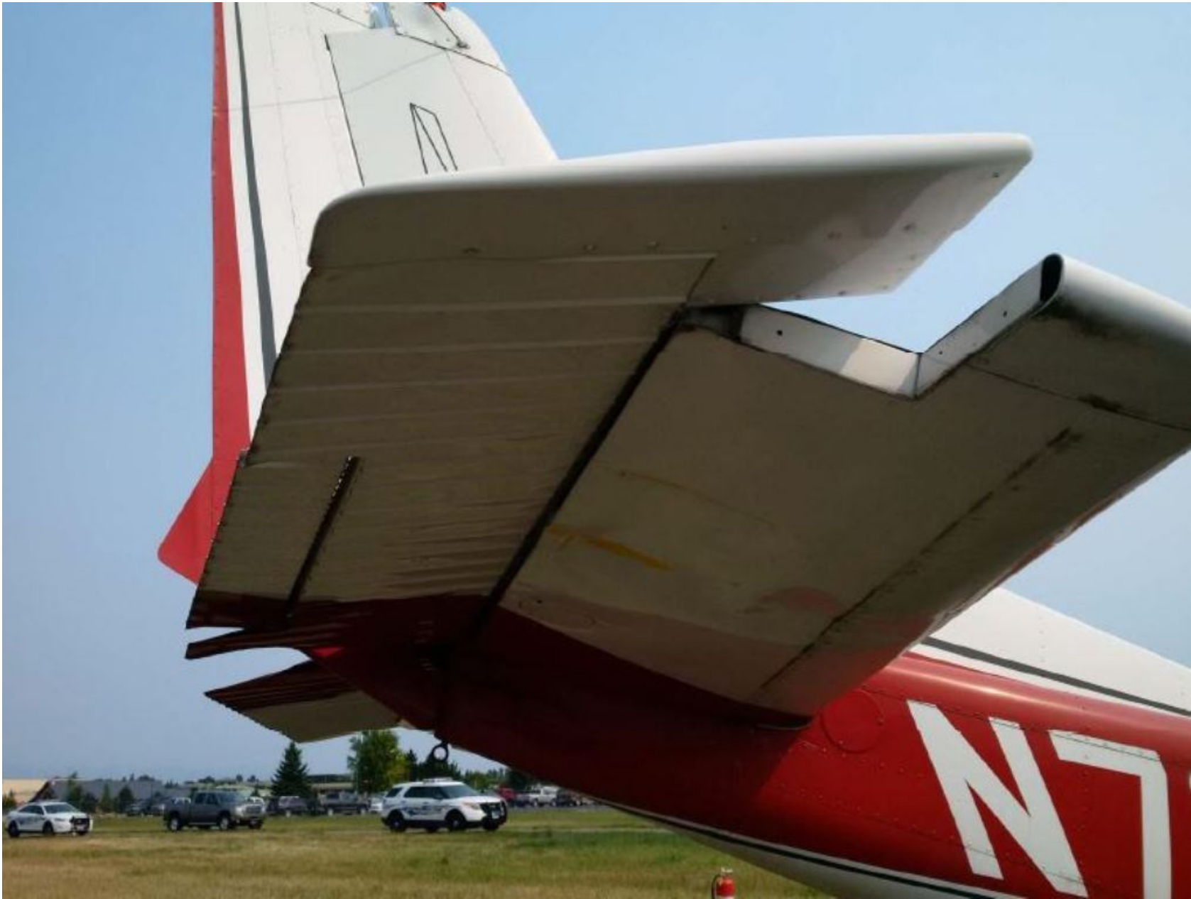
Photo 2 – View of substantial damage to horizontal stabilizer (Courtesy of FAA)
