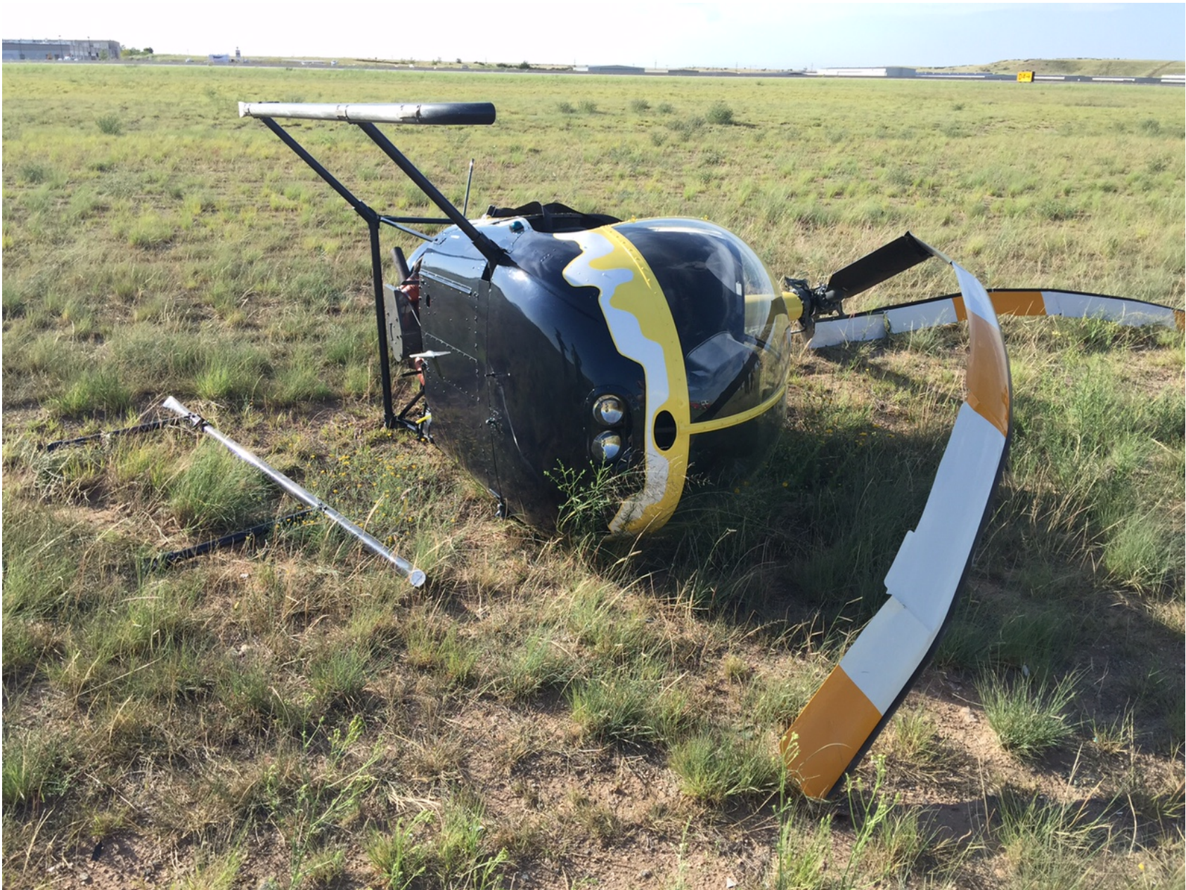
Photo 1 – View of main rotor damage (photo courtesy of the FAA)
