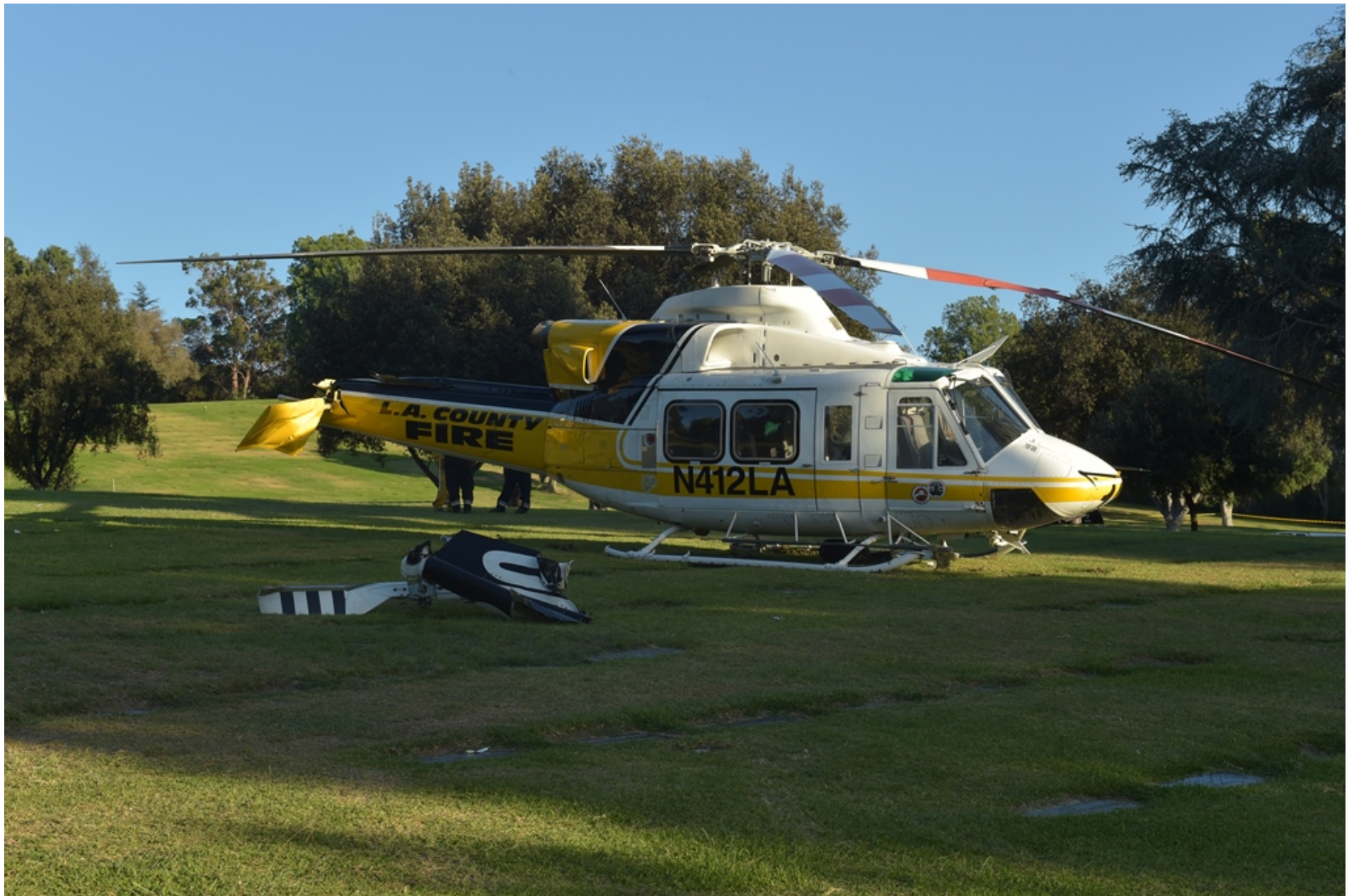
Photo 1 – View of substantial damage to tail pylon, main rotor and tail rotor blades
