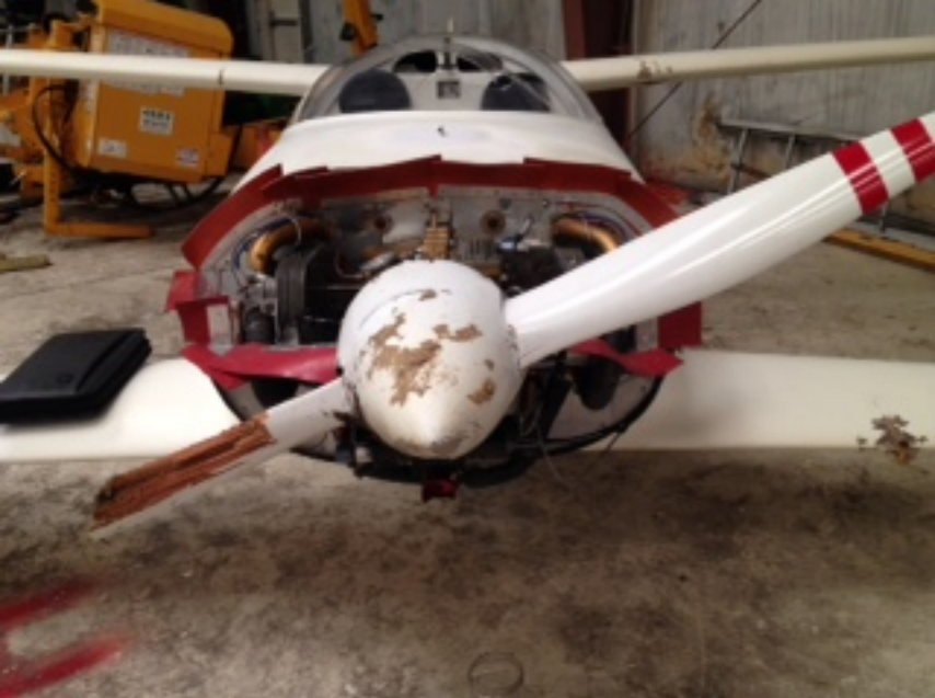
Photo 1-View of substantial damage to left main wing (Photo courtesy of the FAA)
