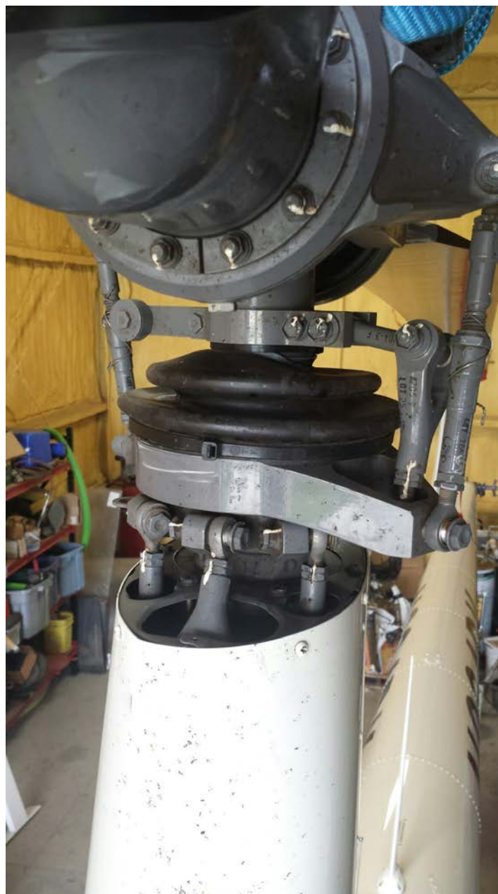
Photo 2 - View of fork assembly and upper arm damage (photo courtesy of the pilot)
