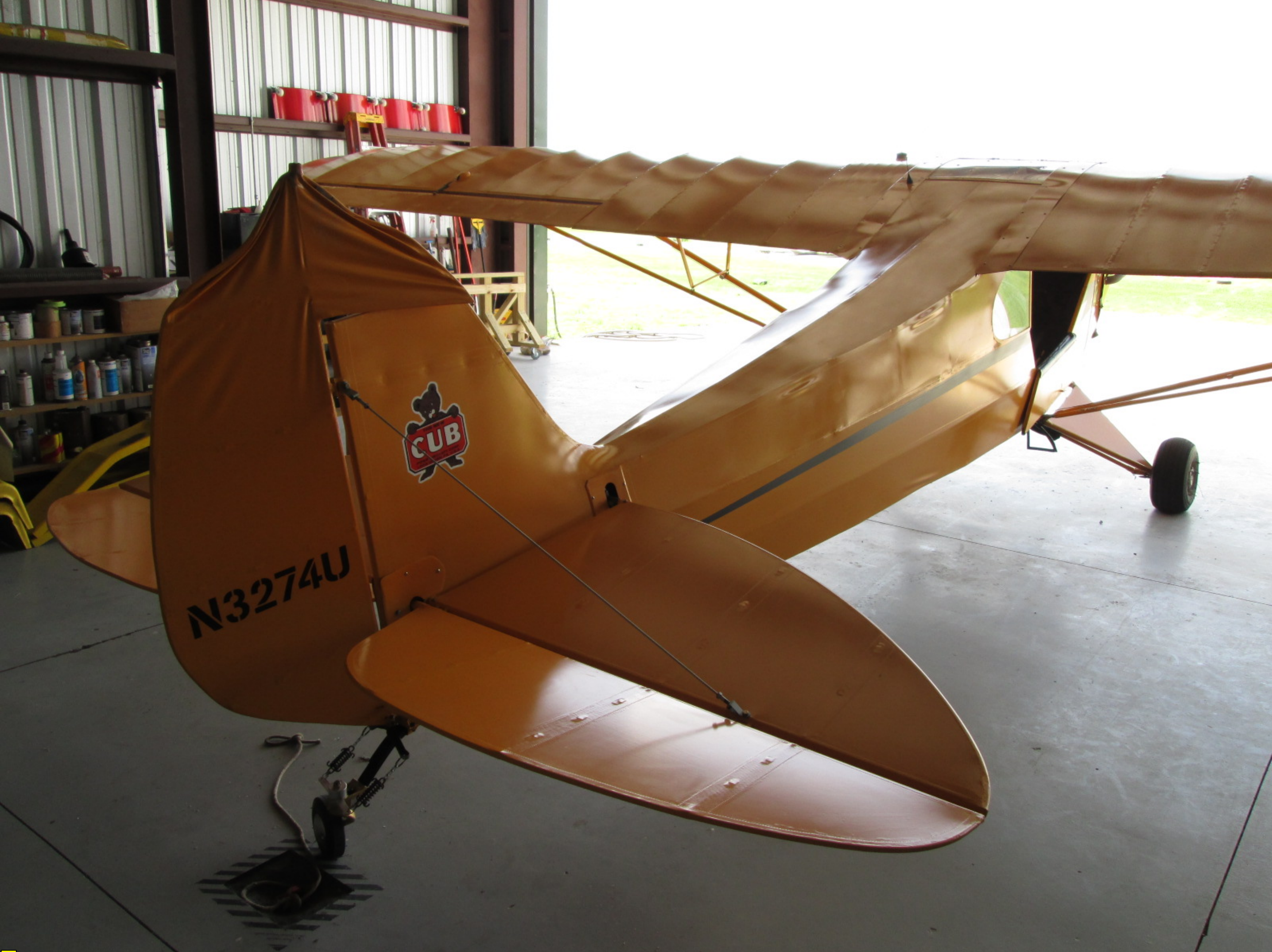
Photograph 1: Substantial damage to empennage (Courtesy of FAA)
