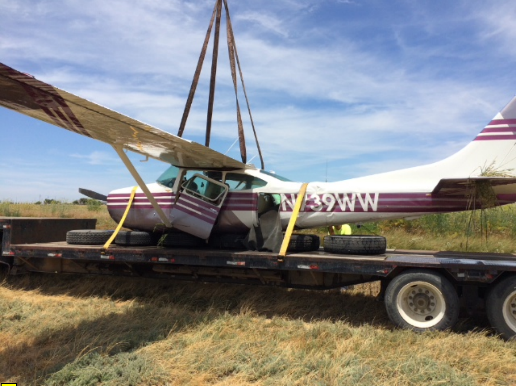
Photo 2 – Fuselage Damage from Left Aft (photo courtesy of owner)
