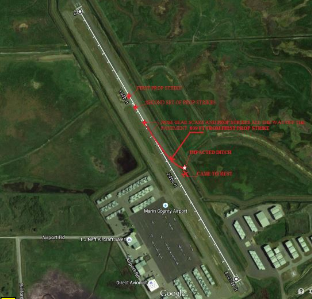
Photo 1: Wreckage Path Diagram (Courtesy of FAA)
