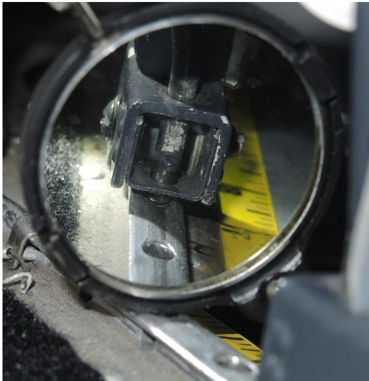
Textron Aviation photograph "Wreckage exam ASI-15-BQ-029.jpg" showing adjustment pin not engaging in seat rail.
