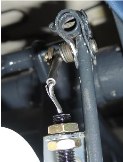
Textron Aviation photograph “Wreckage exam ASI-15-BQ-021.JPG” showing washer stack.
