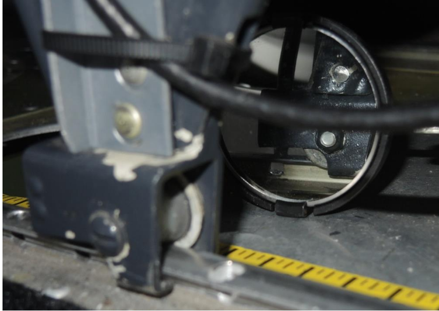
Textron Aviation photograph "Wreckage exam ASI-15-BQ-028.jpg" showing adjustment pin not engaging in seat rail.
