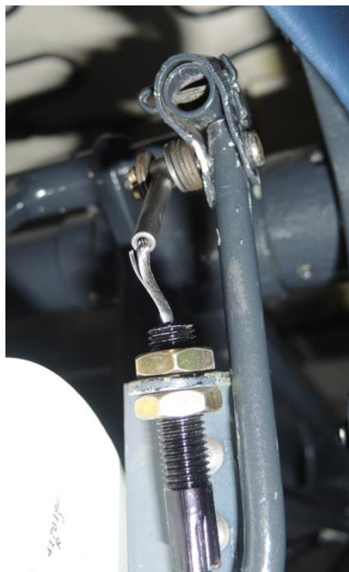
Textron Aviation photograph "Wreckage exam ASI-15-BQ-021.jpg" showing seat adjustment pin sitting against S2300-26. Camera is looking aft and right side of photograph is outboard.
