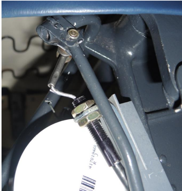
Textron Aviation photograph "Wreckage exam ASI-15-BQ-020.jpg" showing installation of 1299377-20 and S2300-26. Camera is looking inboard and left side of photograph is forward.
