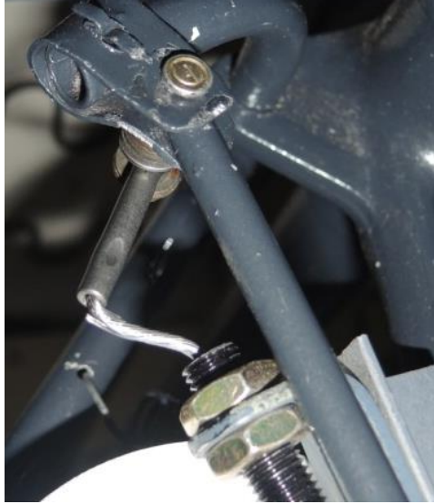
Textron Aviation photograph "Wreckage exam ASI-15-BQ-020.jpg" showing double bend in cable and two separated cable strands at base of terminal end. Camera is looking inboard and left side of photograph is forward.
