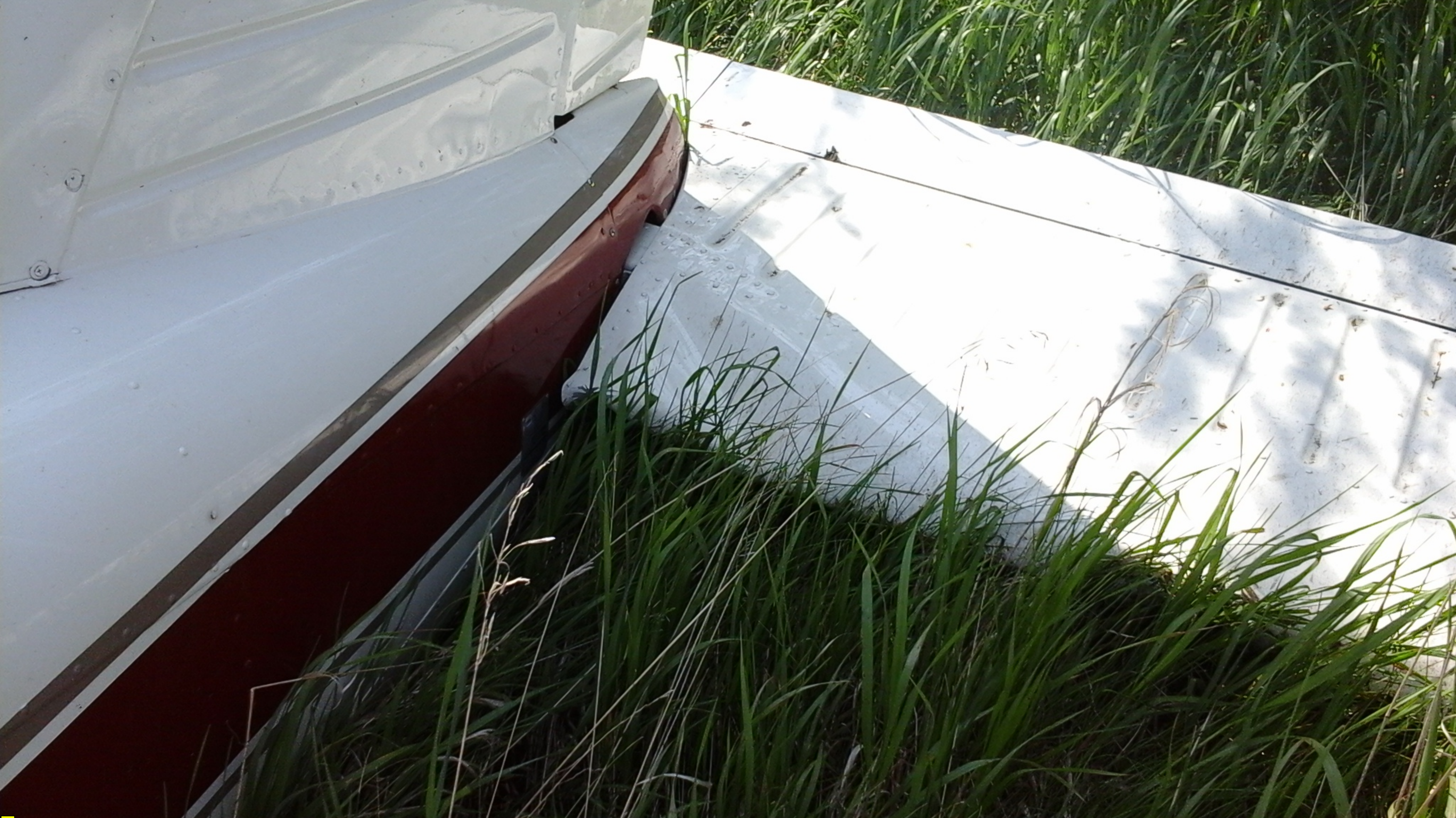
Photograph 2: Substantial damage to airplane left side horizontal stabilizer (Courtesy of FAA)
