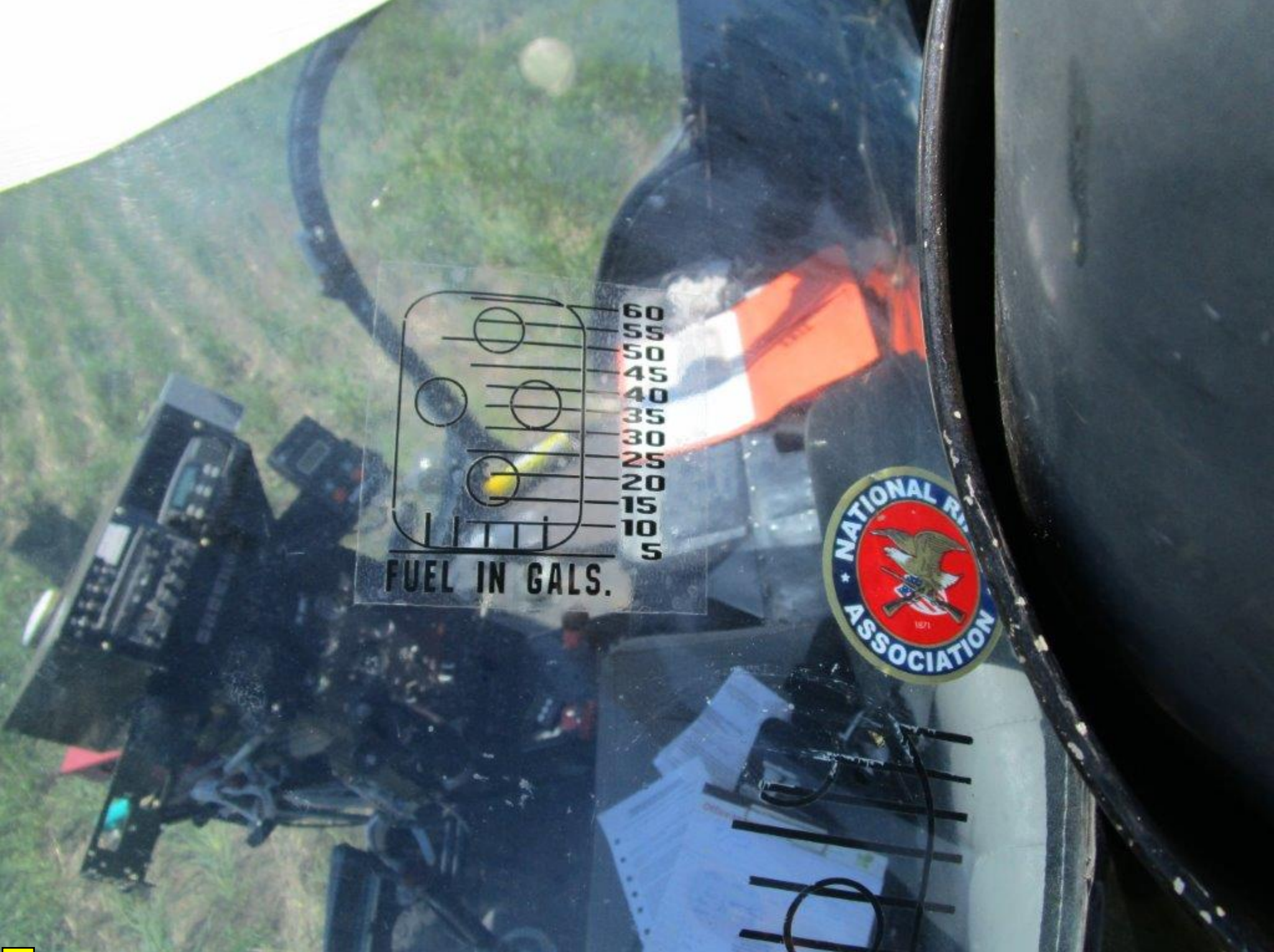
Photo 4 – Fuel Placard (Courtesy of FAA)
