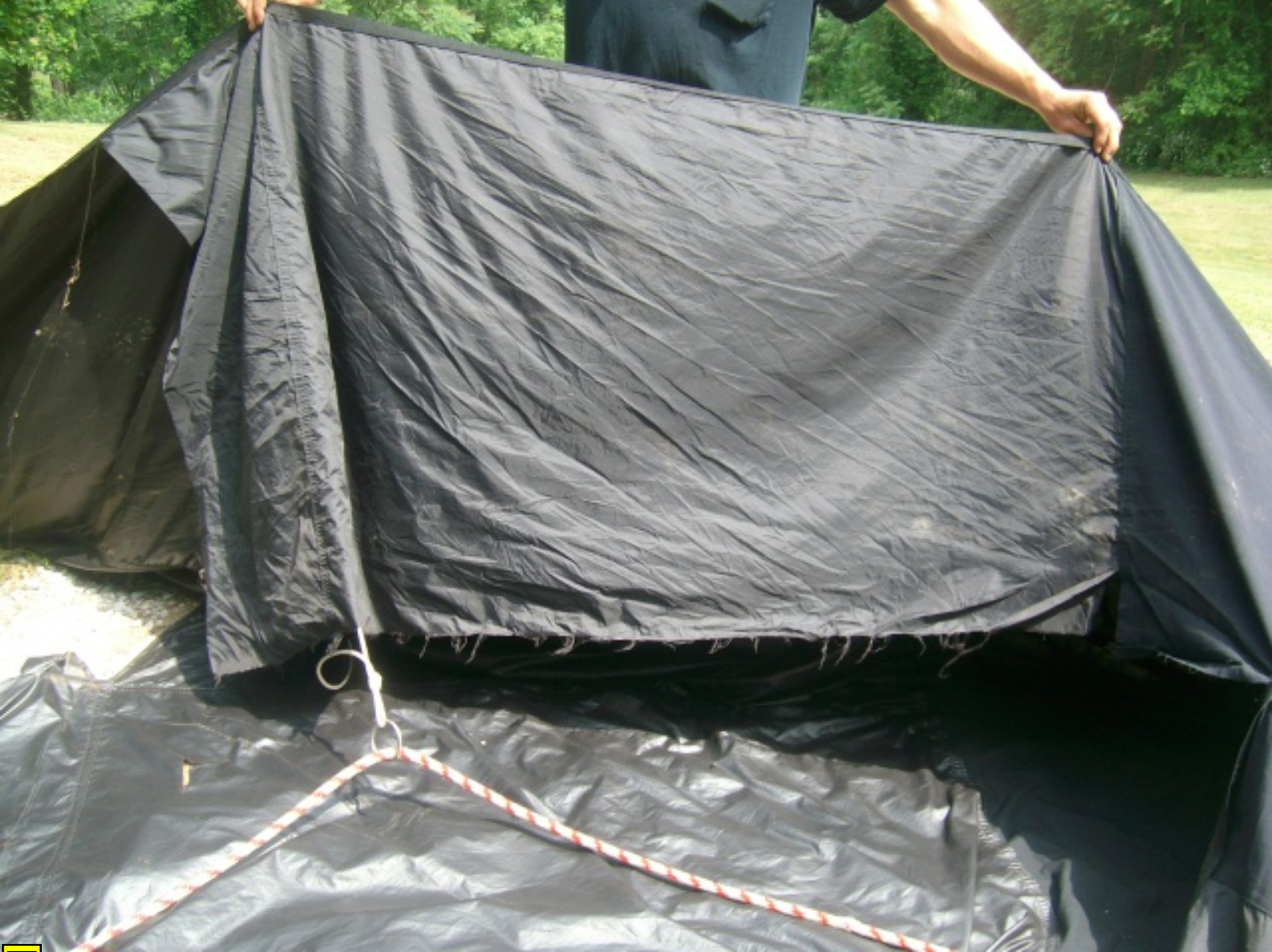
Photograph 3: Substantial Damage to Balloon Tiles (Courtesy of Pilot)
