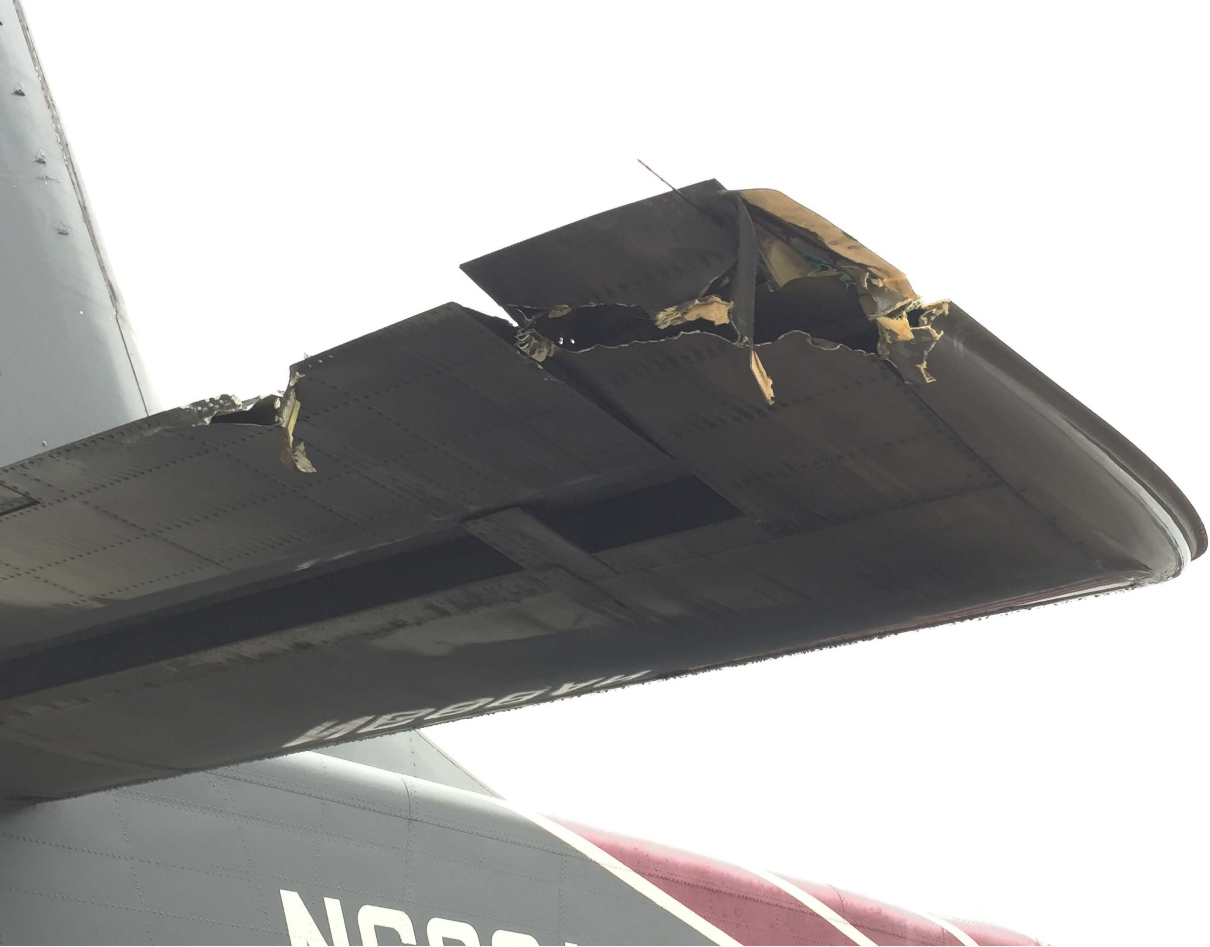
Photo 2 - Horizontal Stabilizer (Photo Courtesy of Operator)
