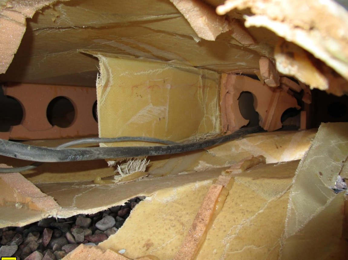
Photo 2 – Right Wing spar Damage (Photo Courtesy of FAA)
