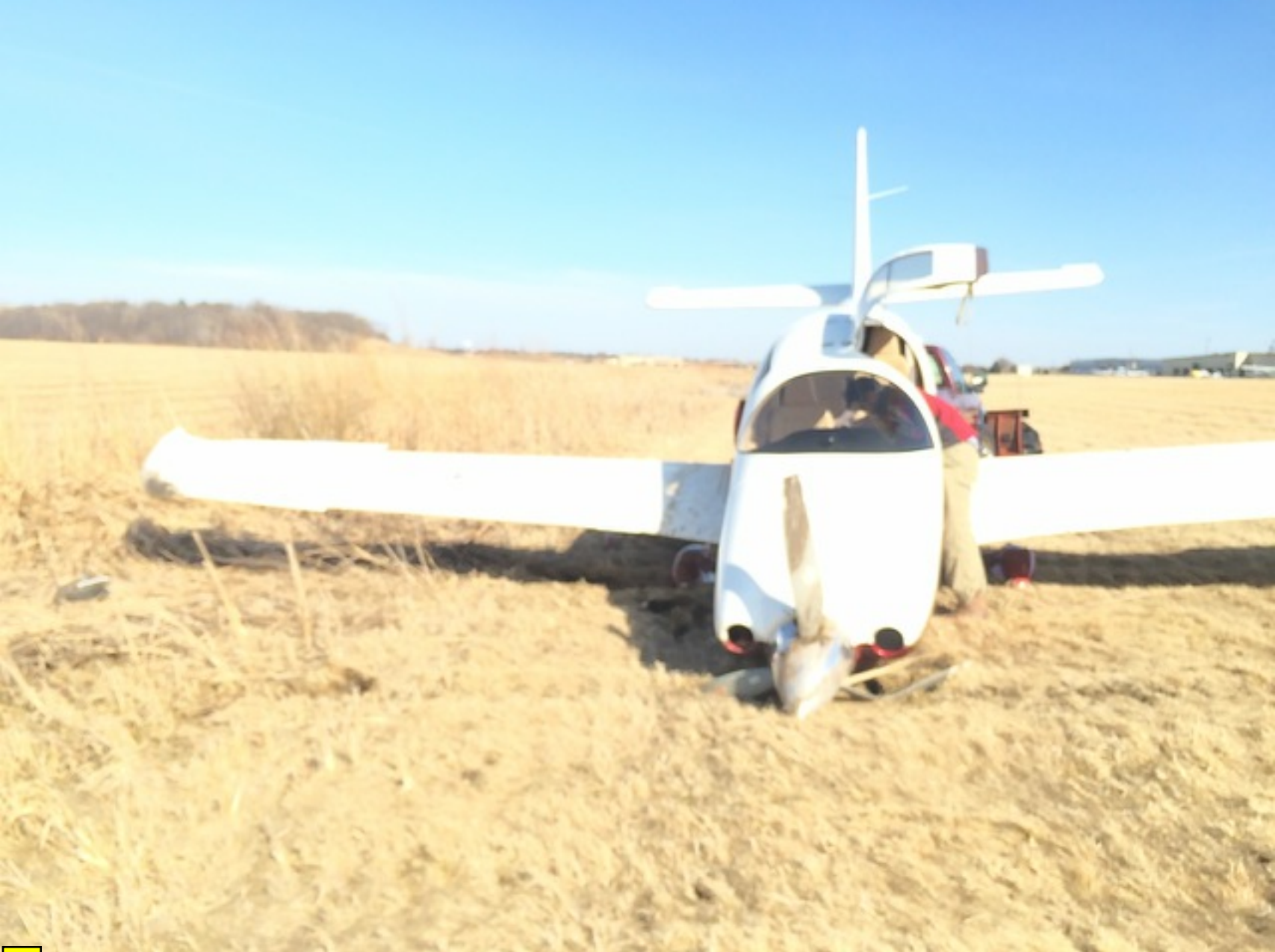
Photo 3 – Airplane with Collapsed Nose Gear (Photo courtesy of FAA)
