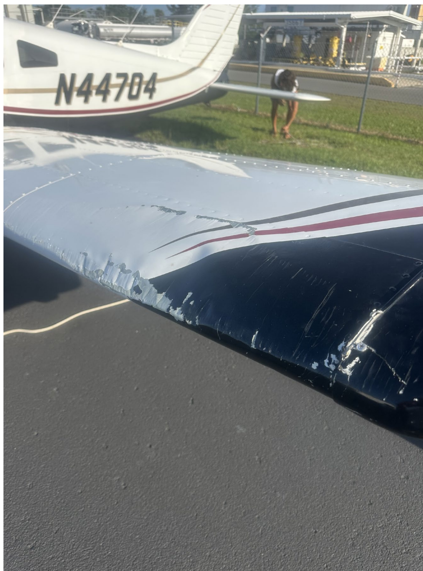
Photograph 1 - left wing damage (Courtesy of FAA)
