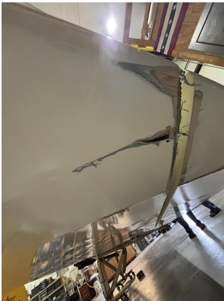
Photograph 2 - View of damage to the lower left wing and aileron. (Courtesy of FAA)
