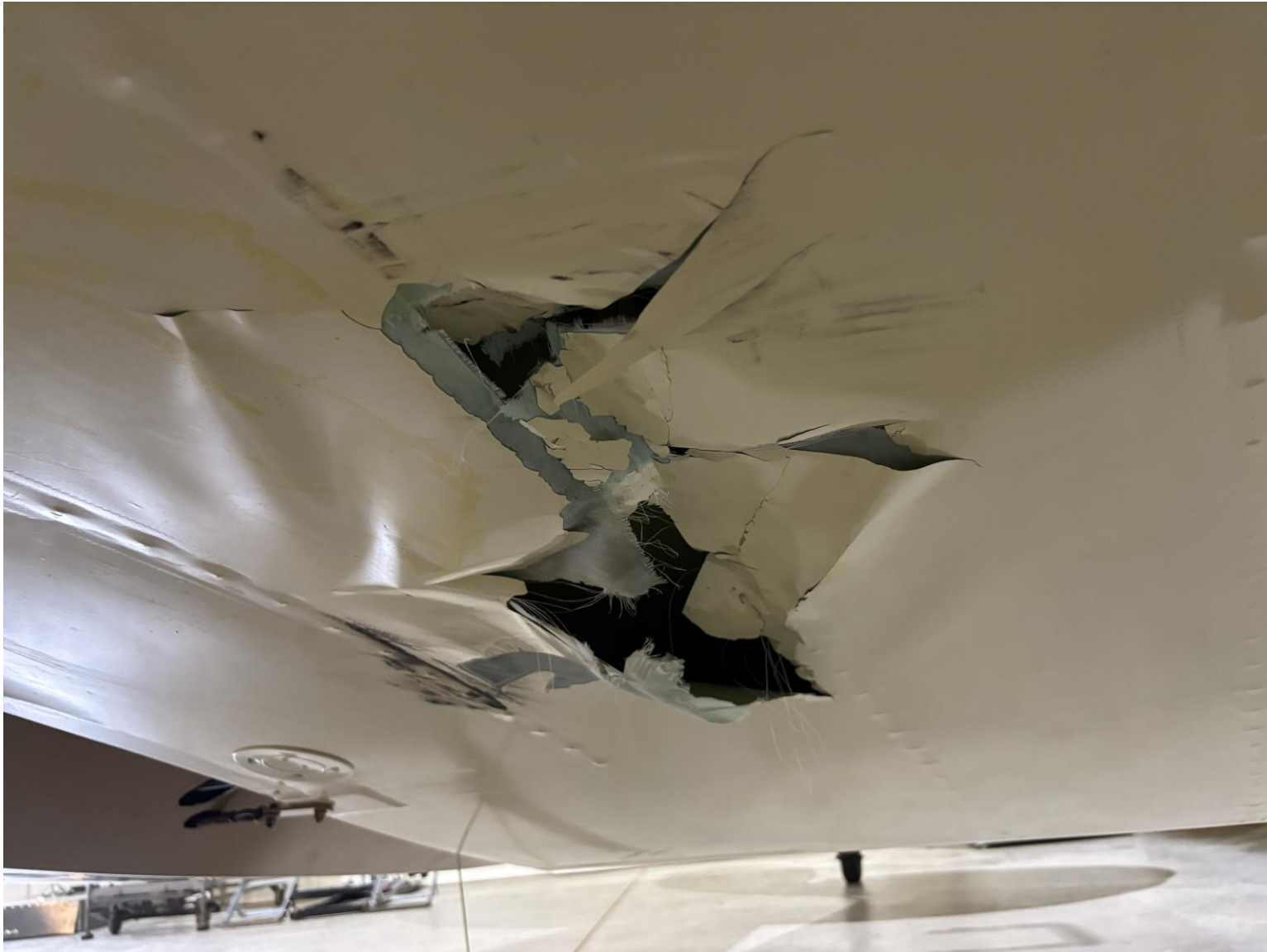
Photograph 3 - View of damage to the lower left wing. (Courtesy of FAA)
