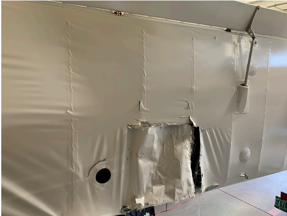
Photograph 2 - Damage to left wing (Courtesy of Pilot)
