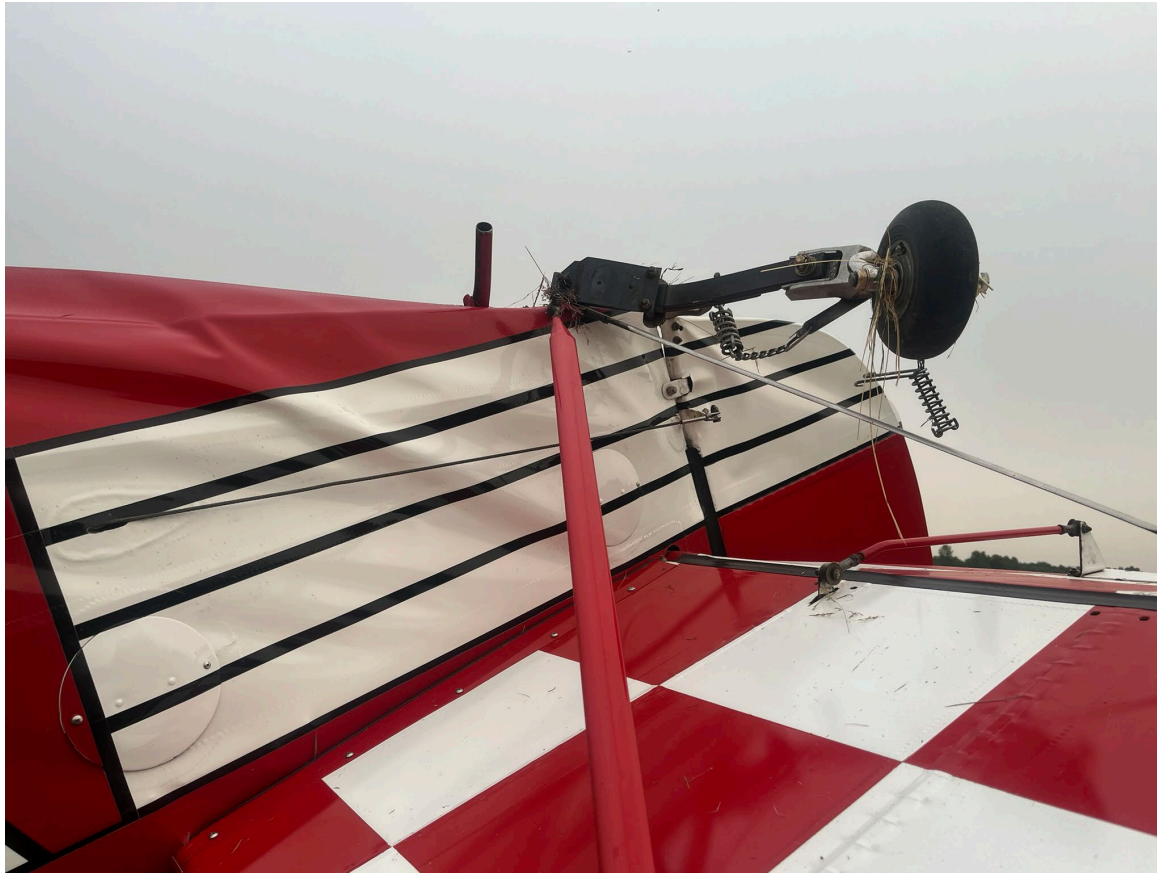
Photograph 2 - Damage to Empennage (Source: FAA)
