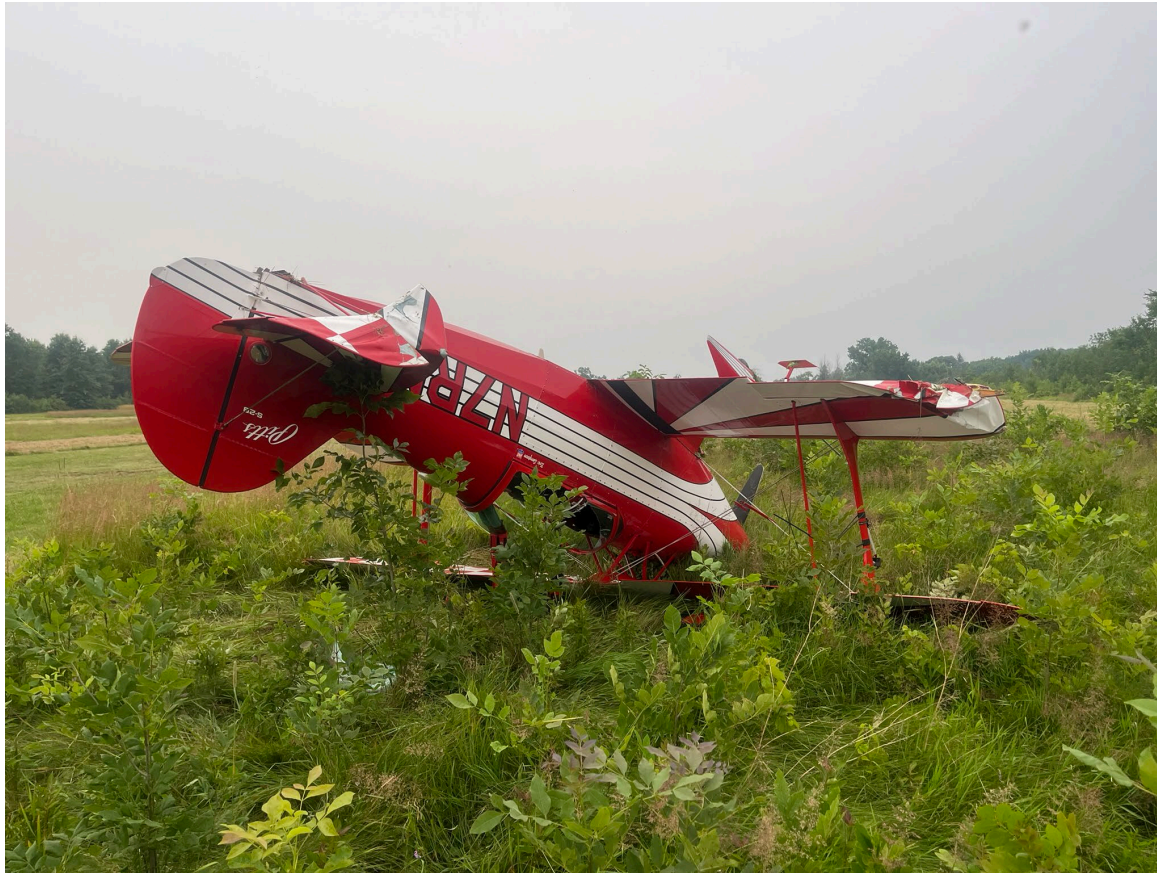
Photograph 3 - Damage to Left Lower Wing and Elevator (Source: FAA)
