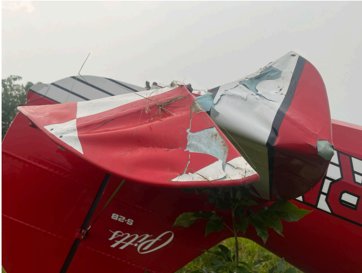
Photograph 4 - Damage to Elevator (Source: FAA)
