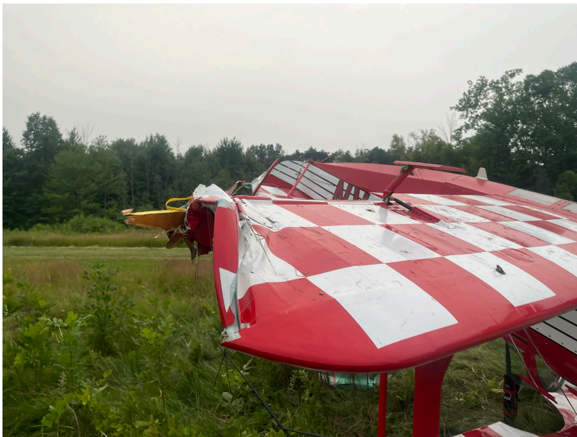
Photograph 5 - Damage to Left Lower Wing (Source: FAA)
