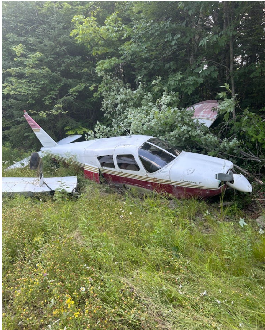
Photograph 1 - View of airplane with separated right wing. (Courtesy of FAA)
