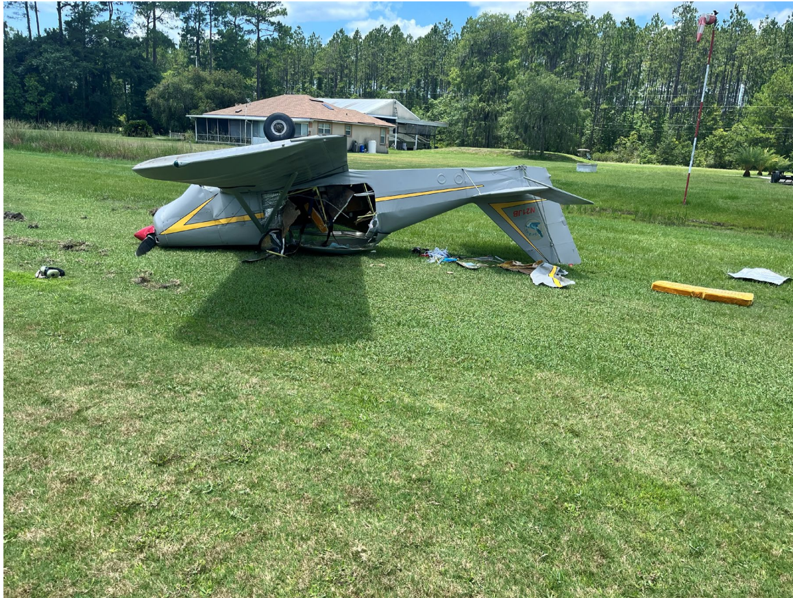
Photograph 1 - Deformation noted to aft fuselage. (Courtesy of FAA)
