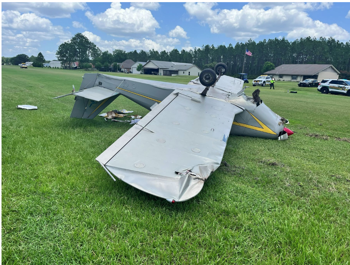
Photograph 2 - Deformation noted to fuselage and left wing. (Courtesy of FAA)
