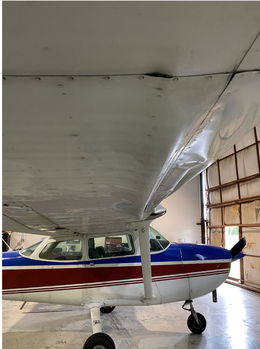
Photograph 1 - Right wing leading edge damage (Courtesy of FAA)
