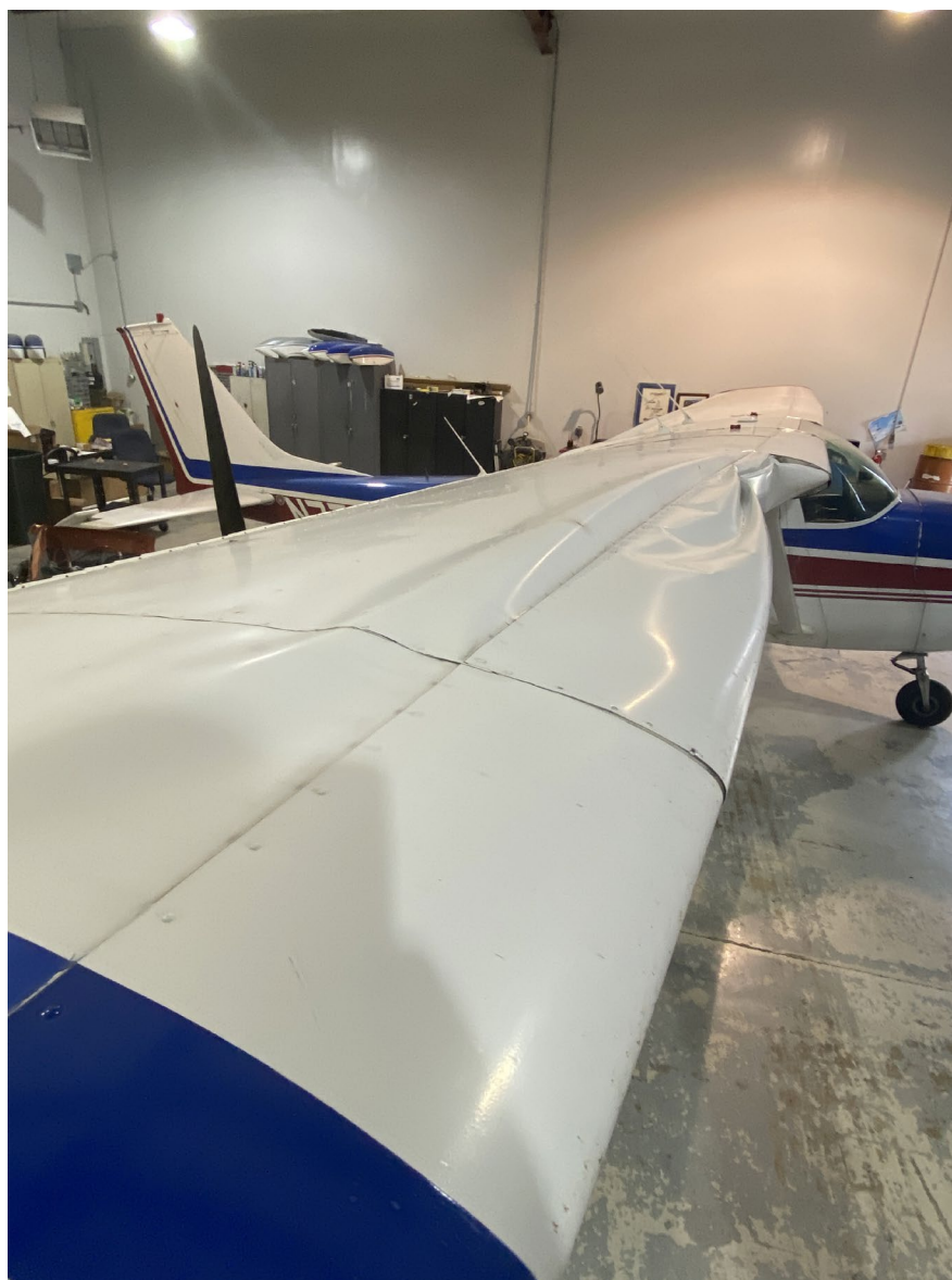
Photograph 2 -Right wing leading edge damage (Courtesy of FAA)
