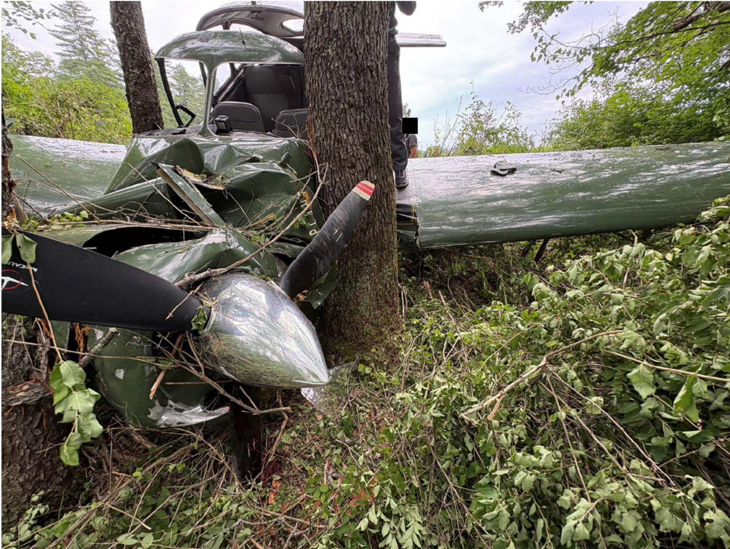
Photograph 1 - Front of the Airplane On-Scene with Engine Mount, Fuselage, and Right Wing Damage
