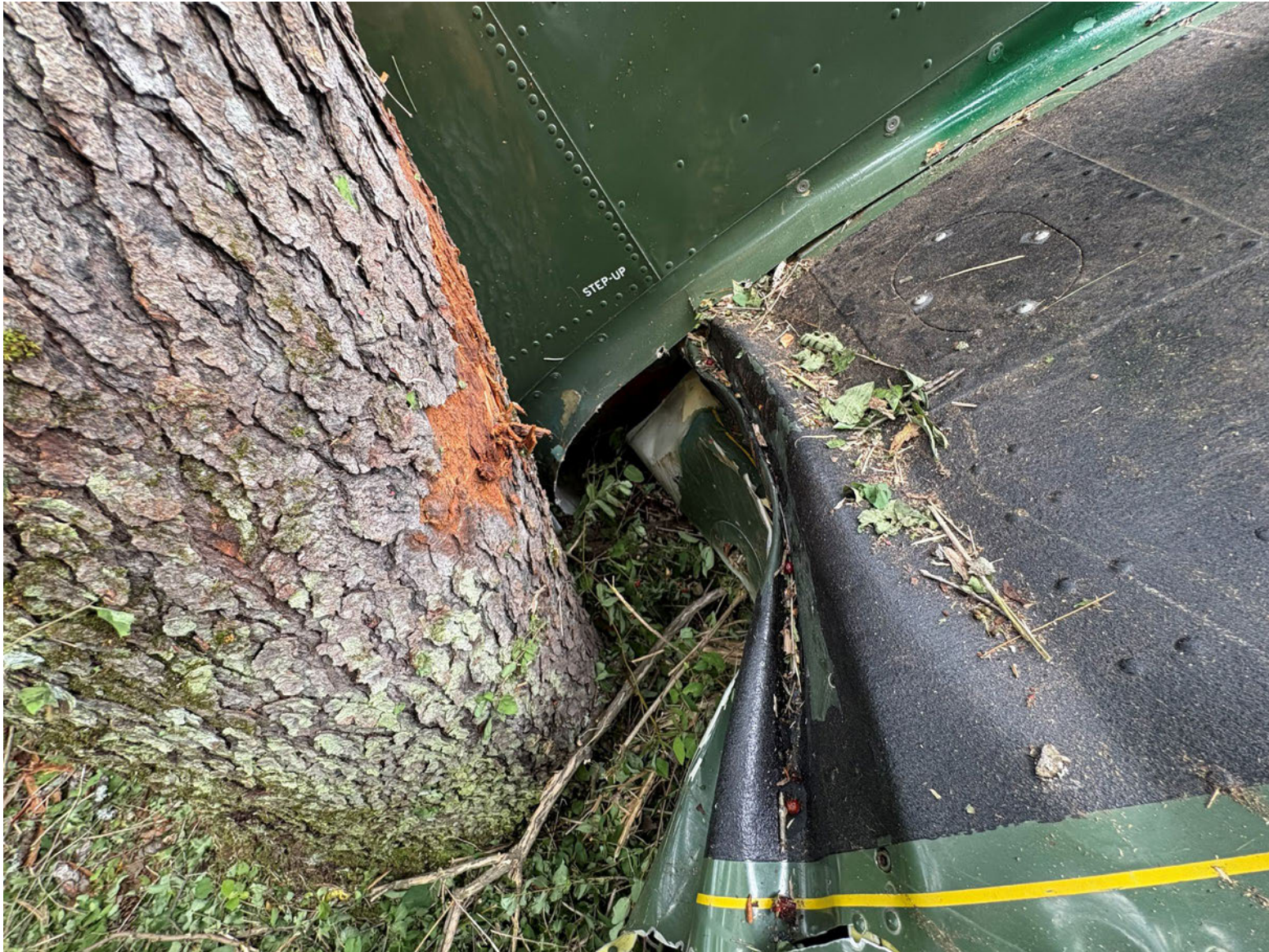
Photograph 2 - Right Wing Forward Inboard Damage
