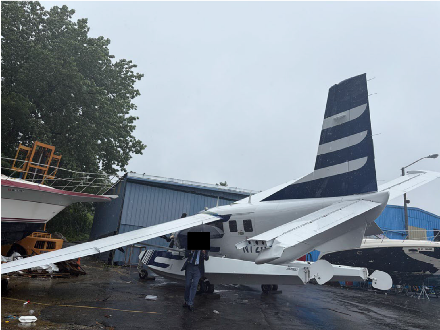
Photograph 2 - Left Elevator Damage (Courtesy of FAA)
