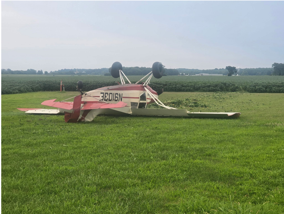
Photograph 2 - Close up of Inverted Airplane Showing Damage to Vertical Fin, Rudder and Wing Struts (Courtesy of FAA)
