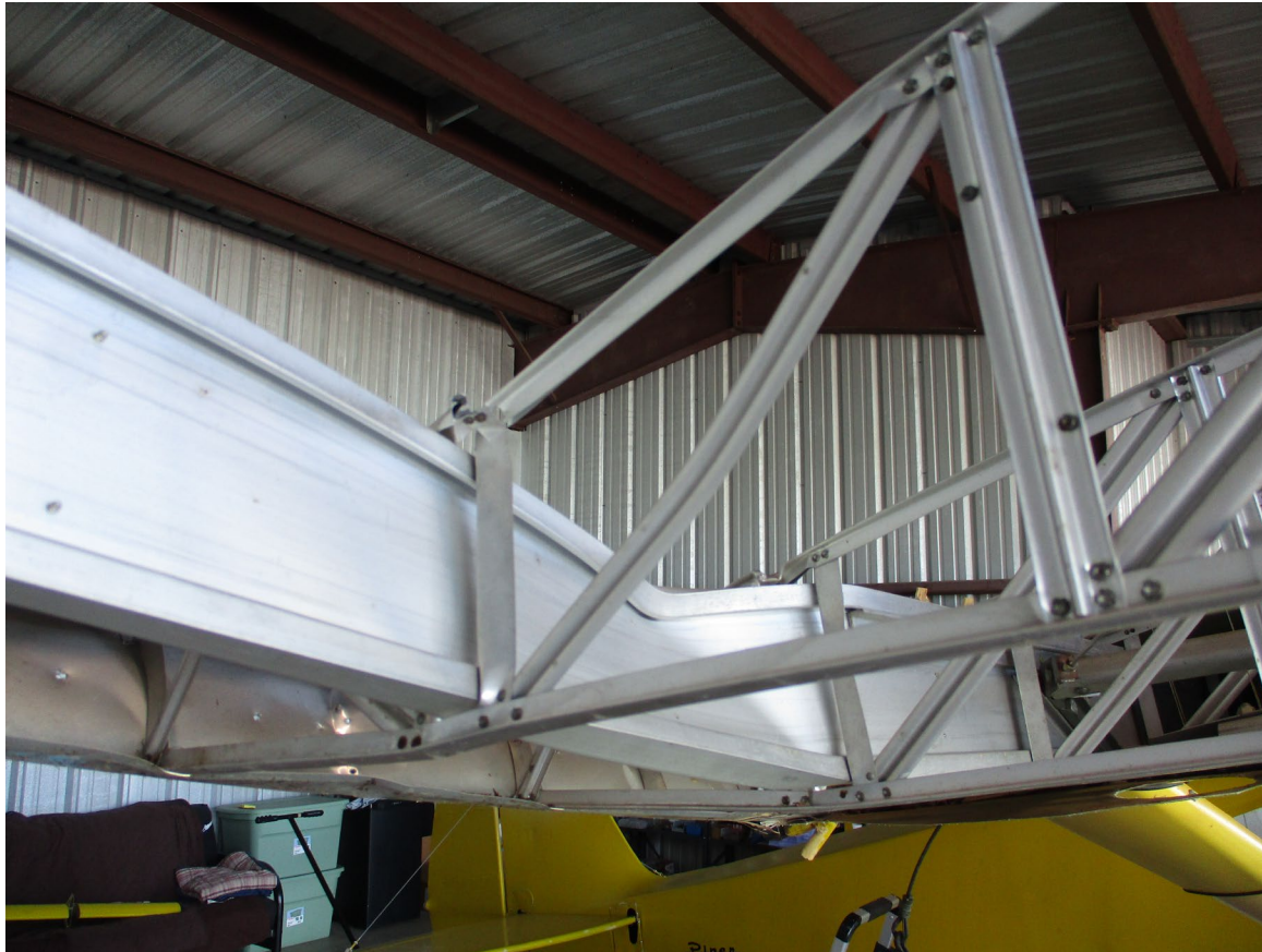
Photograph 2 - Close up of bent spar. (Courtesy of FAA)
