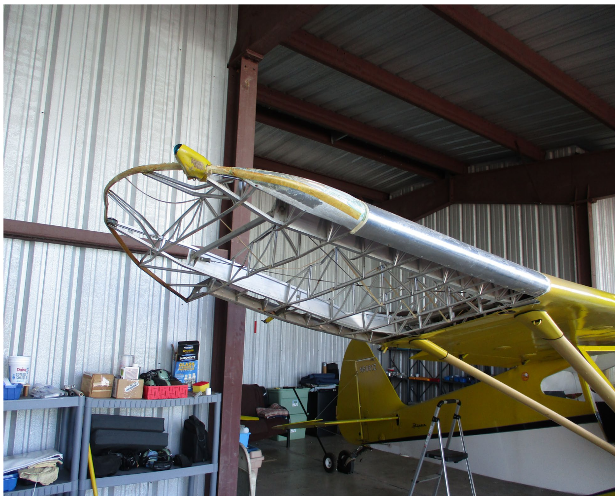
Photograph 1 - View of outboard right-wing spar. (Courtesy of FAA)
