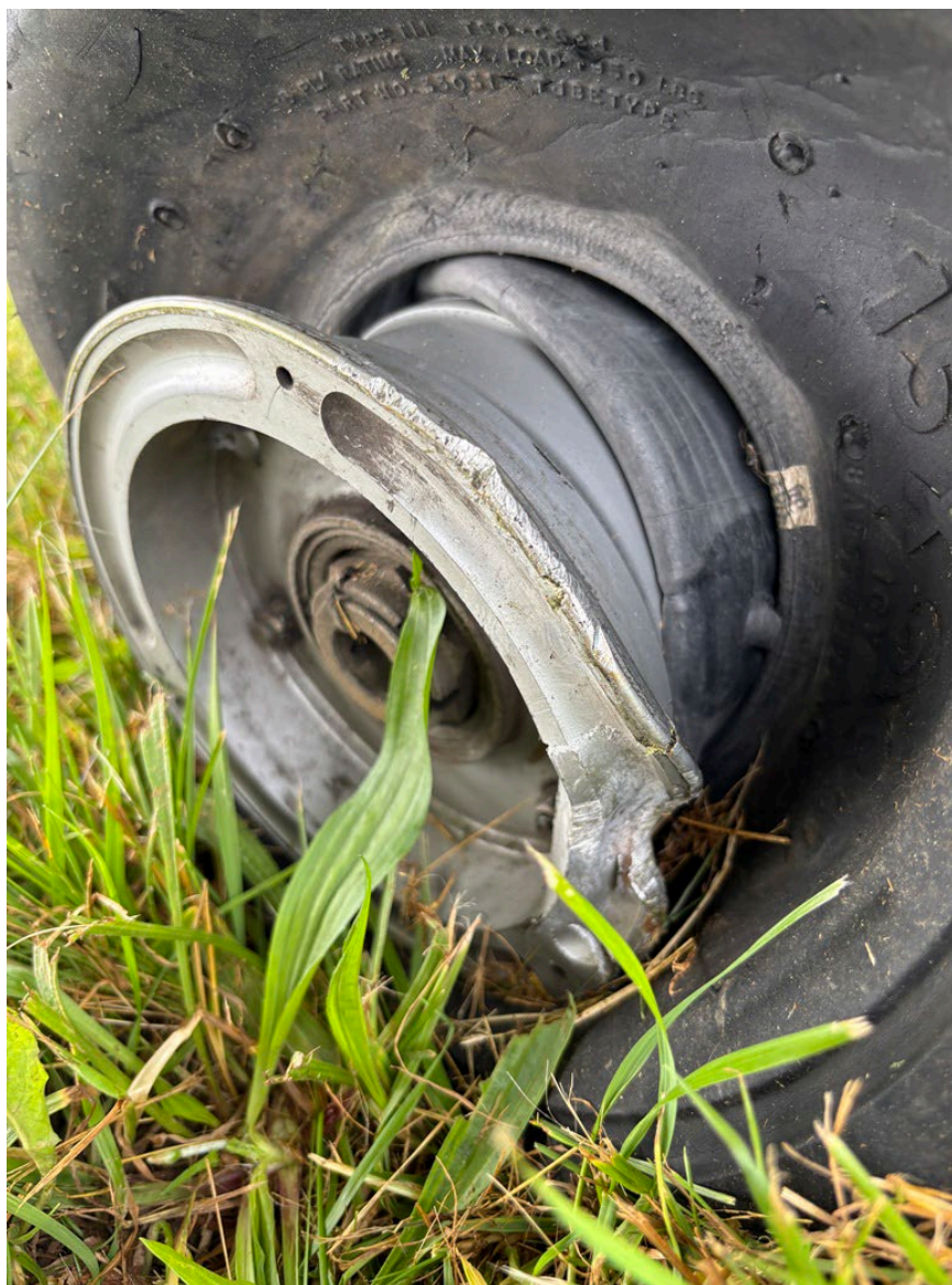
Photograph 7 - Left Main Landing Gear Rim Damage And Deflated Tire (Courtesy of FAA)
