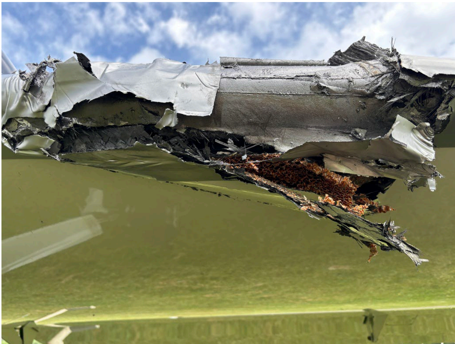
Photograph 9 - Underside View of Composite Left Wing Damage (Courtesy of FAA)
