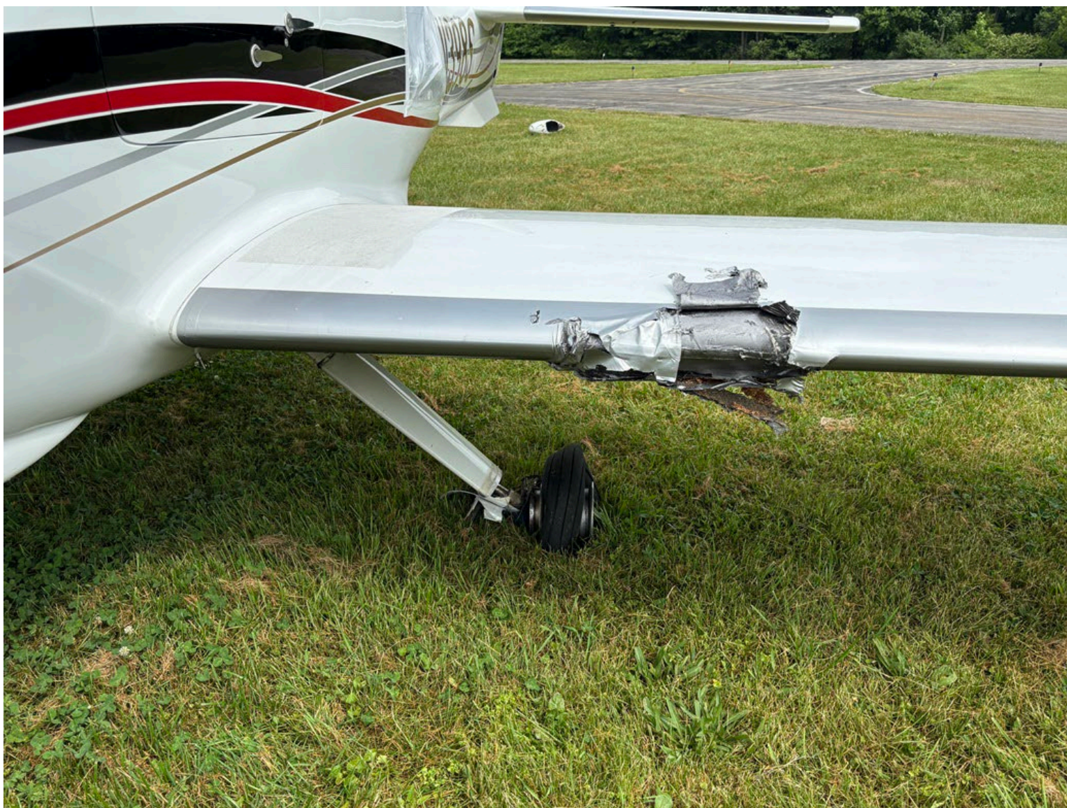
Photograph 8 - Composite Left Wing Damage (Courtesy of FAA)
