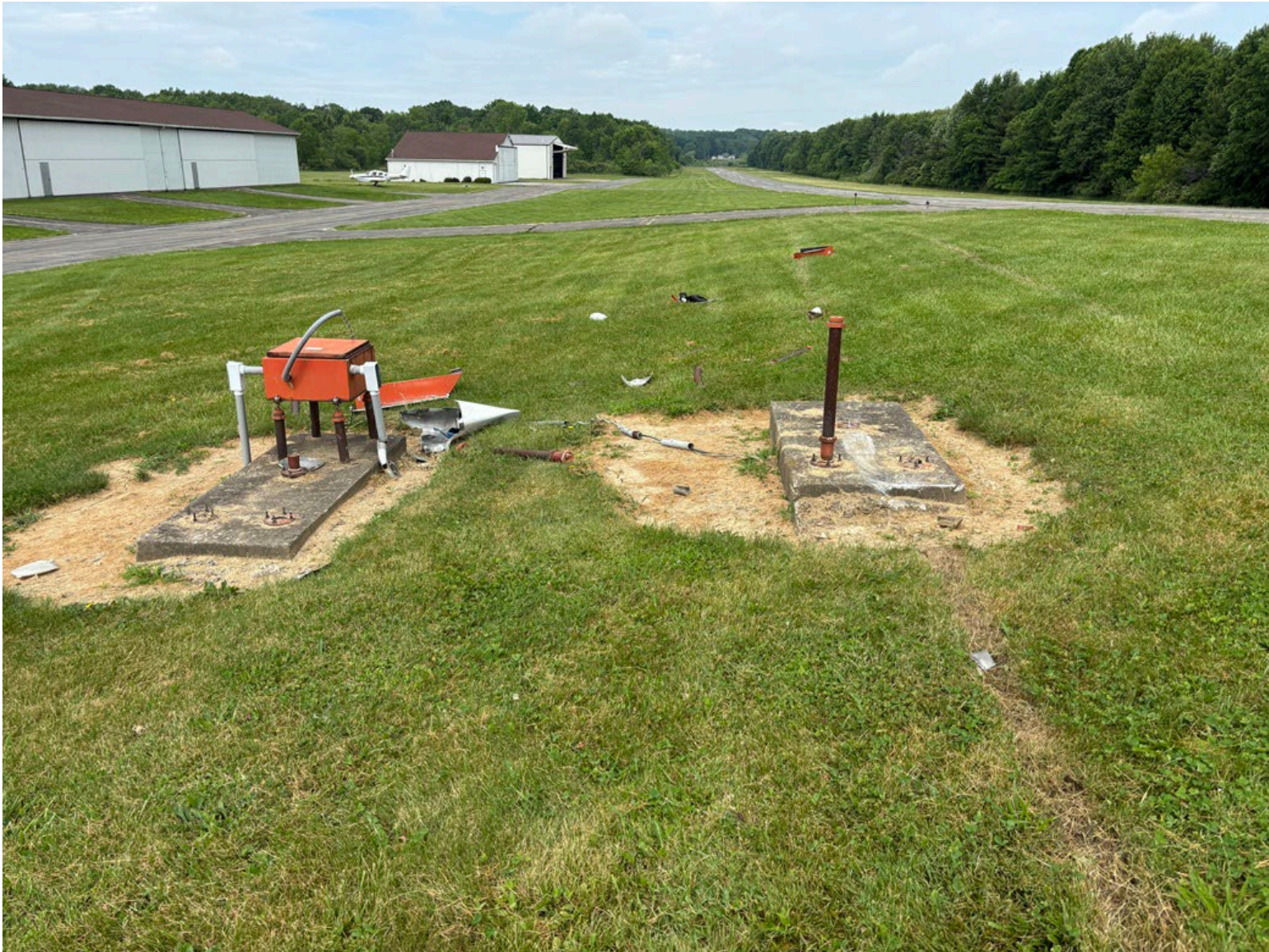
Photograph 6 - Left Main Landing Grass Impression And Contact With VASI Light (Courtesy of FAA)
