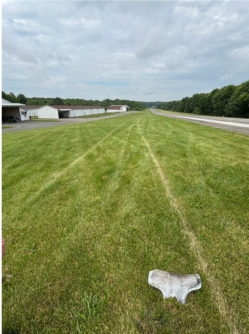
Photograph 3 - Right Main Landing Gear Separated Fairing (Courtesy of FAA)
