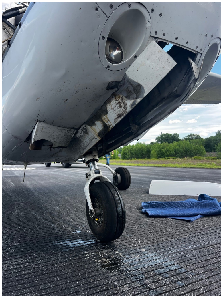
Photograph 1 - Nose landing gear and lower forward fuselage damage (Courtesy of FAA)
