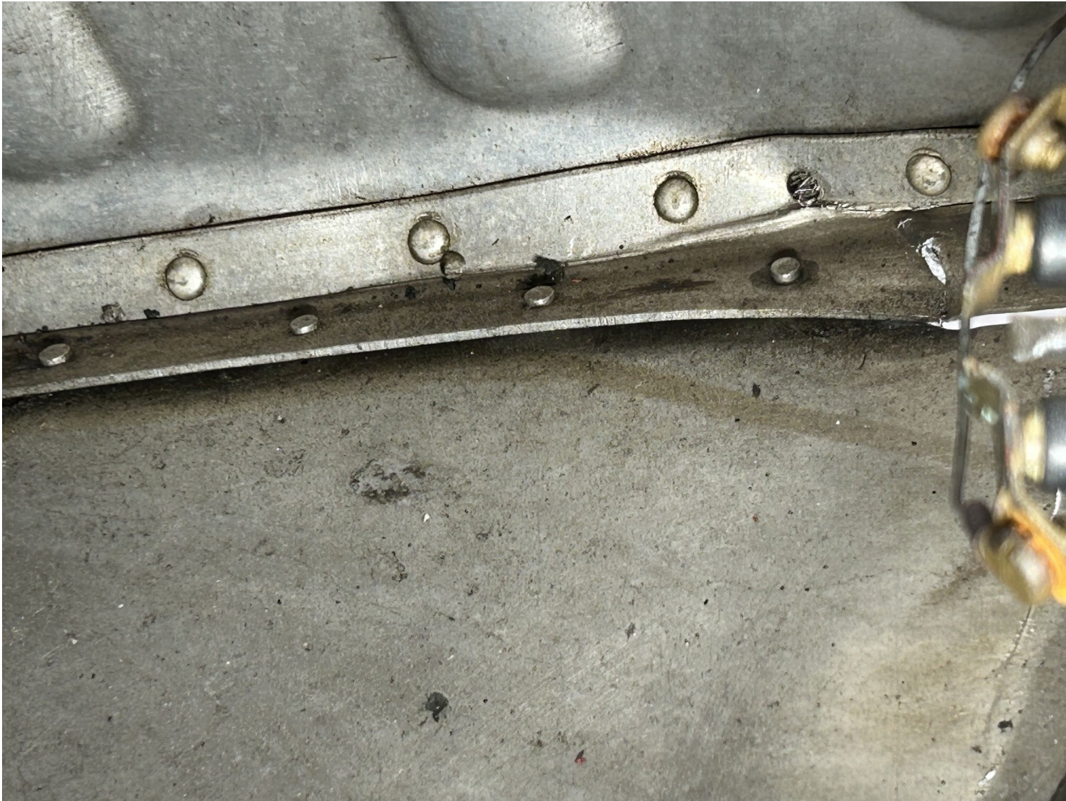
Photograph 3 - Forward fuselage structure damage (Courtesy of FAA)
