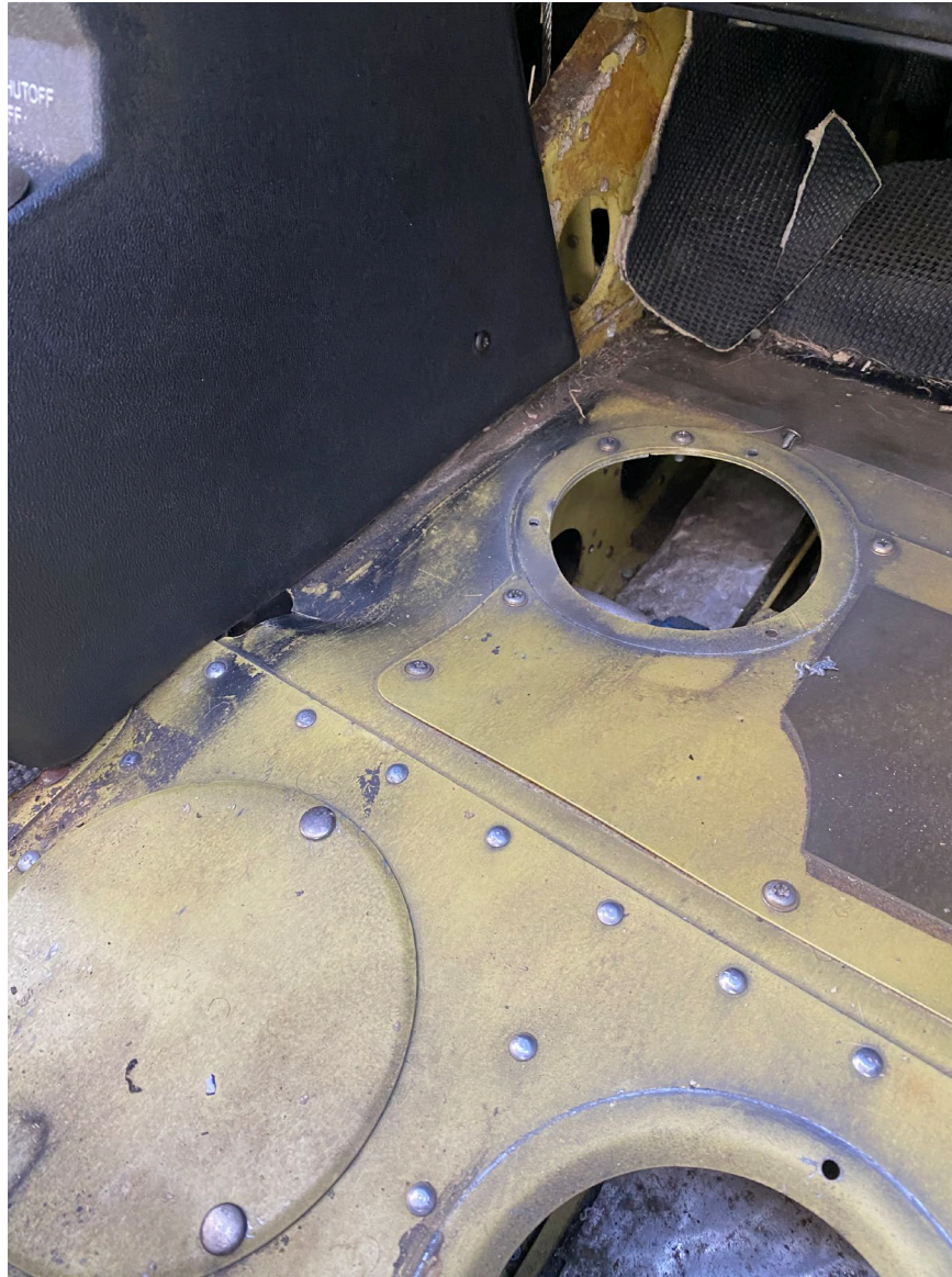
Photograph 2 - Buckling noted to lower right fuselage structure (Courtesy of FAA)
