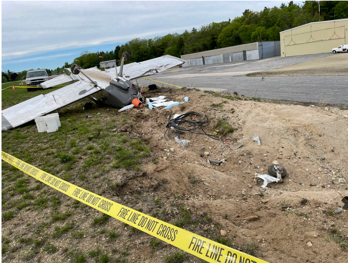
Photograph 1 - View from the nose showing impact point and inverted airplane (Courtesy of FAA)
