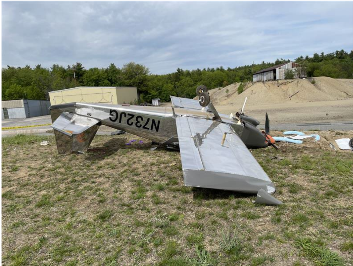
Photograph 3 - Left-hand side view showing damage to empennage (Courtesy of FAA)
