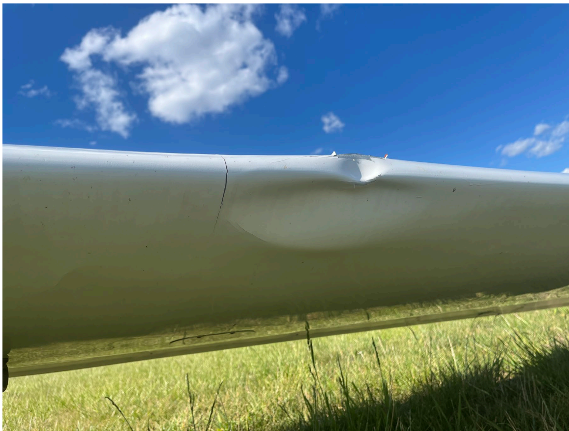
Photograph 2 - Damage to leading edge of left wing (Source: FAA)
