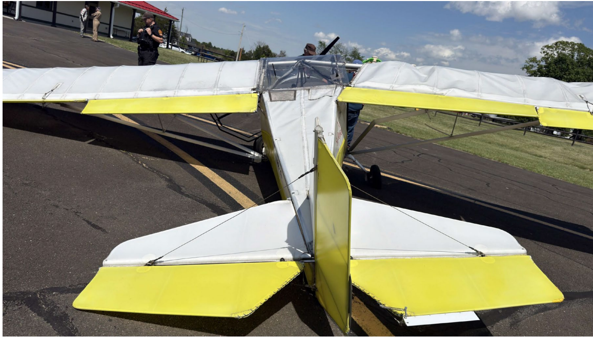
Photograph 1 -Aft view of airplane showing damage to right wing root. (Courtesy of FAA)
