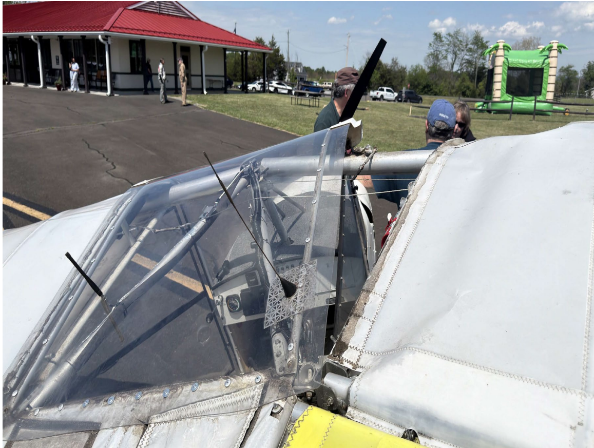
Photograph 2 - Close up view of right damaged wing root. (Courtesy of FAA)
