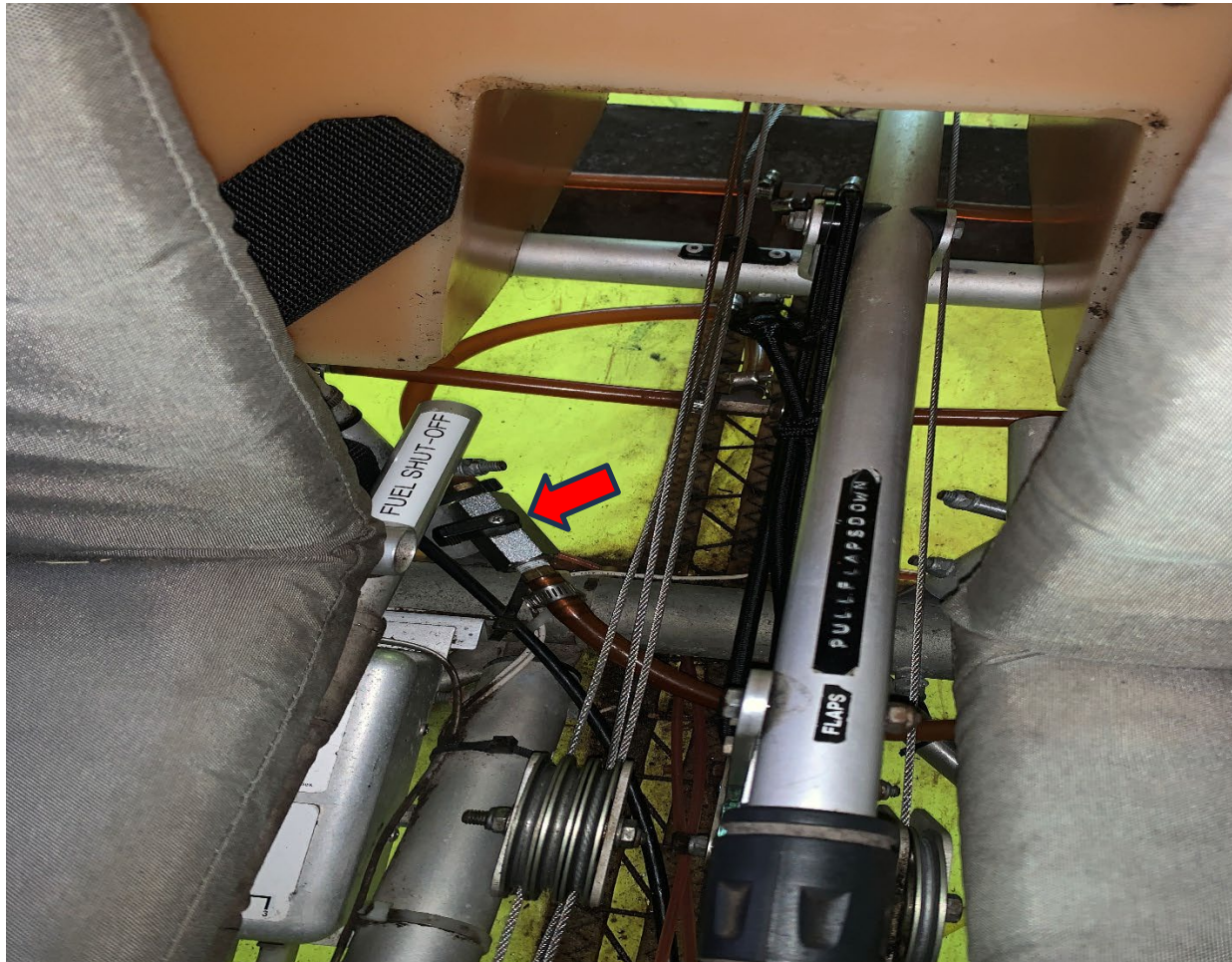
Photograph 3 - View of fuel selector behind seat in the off position. Shown with a red arrow pointing to it. (Courtesy of FAA)
