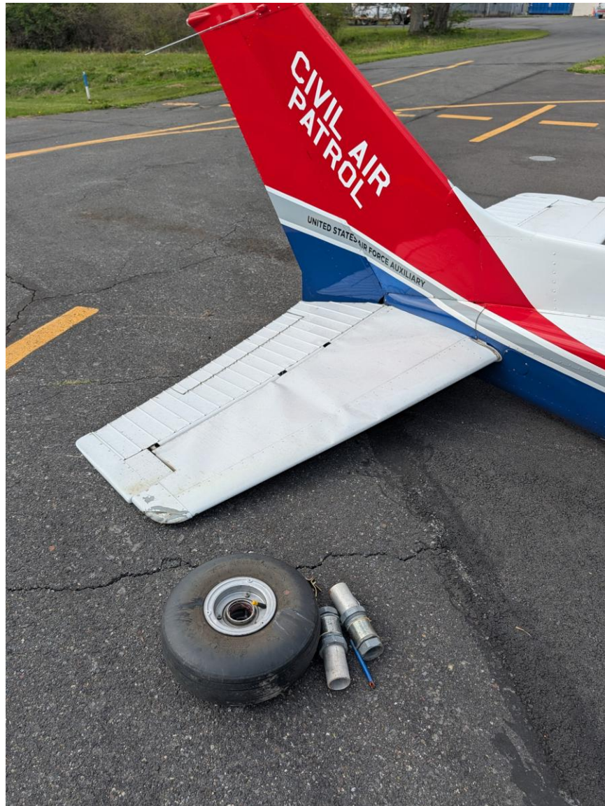
Photograph 3 - View of damage to the right horizontal stabilizer. (Courtesy of FAA)
