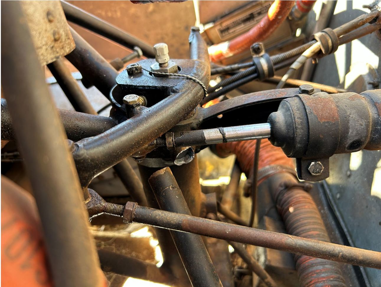
Photograph 3 - View of broken engine mount. (Courtesy of FAA)
