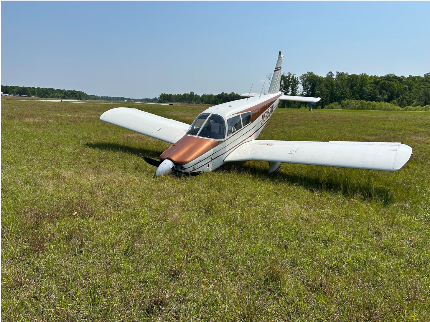
Photograph 2 - Left front view of airplane showing collapsed nose gear. (Courtesy of FAA)
