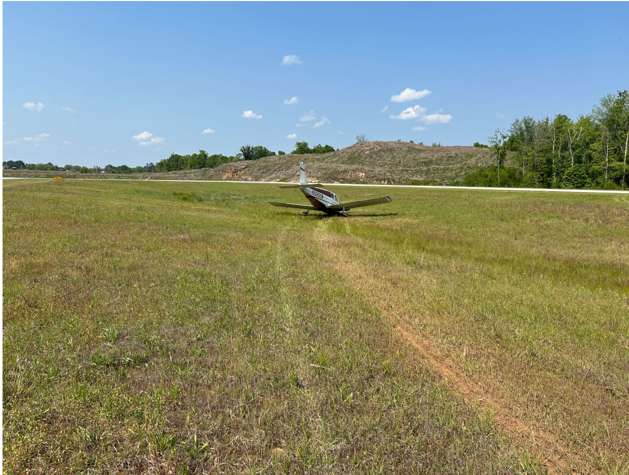
Photograph 1 - Landing gear tracks in the ground leading up to airplane accident location. (Courtesy of FAA)
