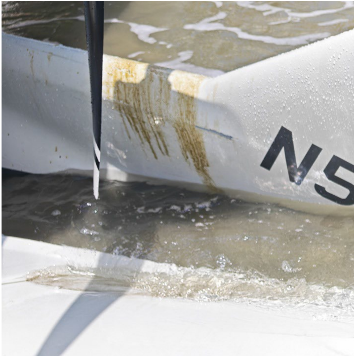
Photograph 2 - Oil Spray (Courtesy of Pilot)
