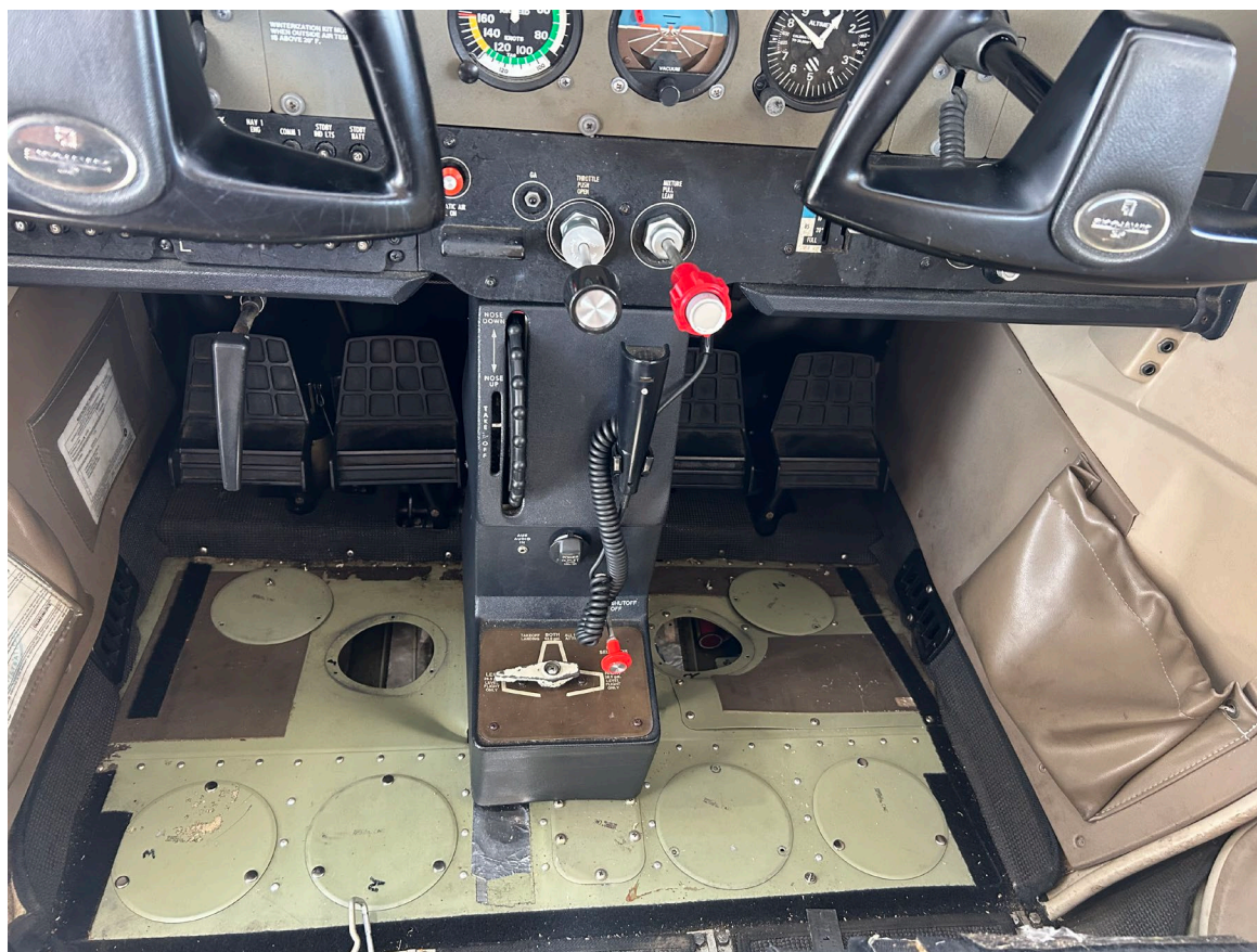
Photograph 1 - Deformation noted to fuselage box structure (Courtesy of Flight School)
