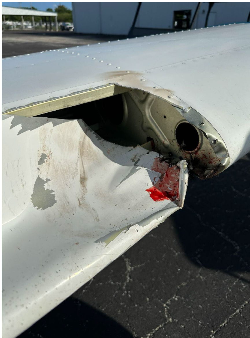
Photograph 1 - Impact Damage (Courtesy of Operator)
