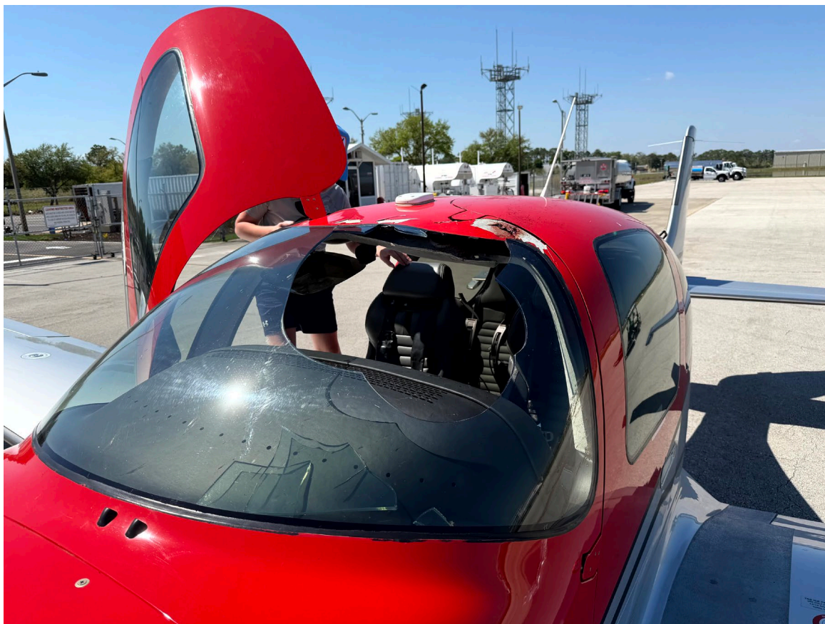
Photograph 1 - Impact damage noted to windshield and roof structure (Courtesy of FAA)
