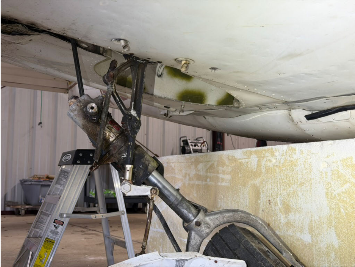
Figure 4: Right main landing gear assembly showing structural separation and damage.
