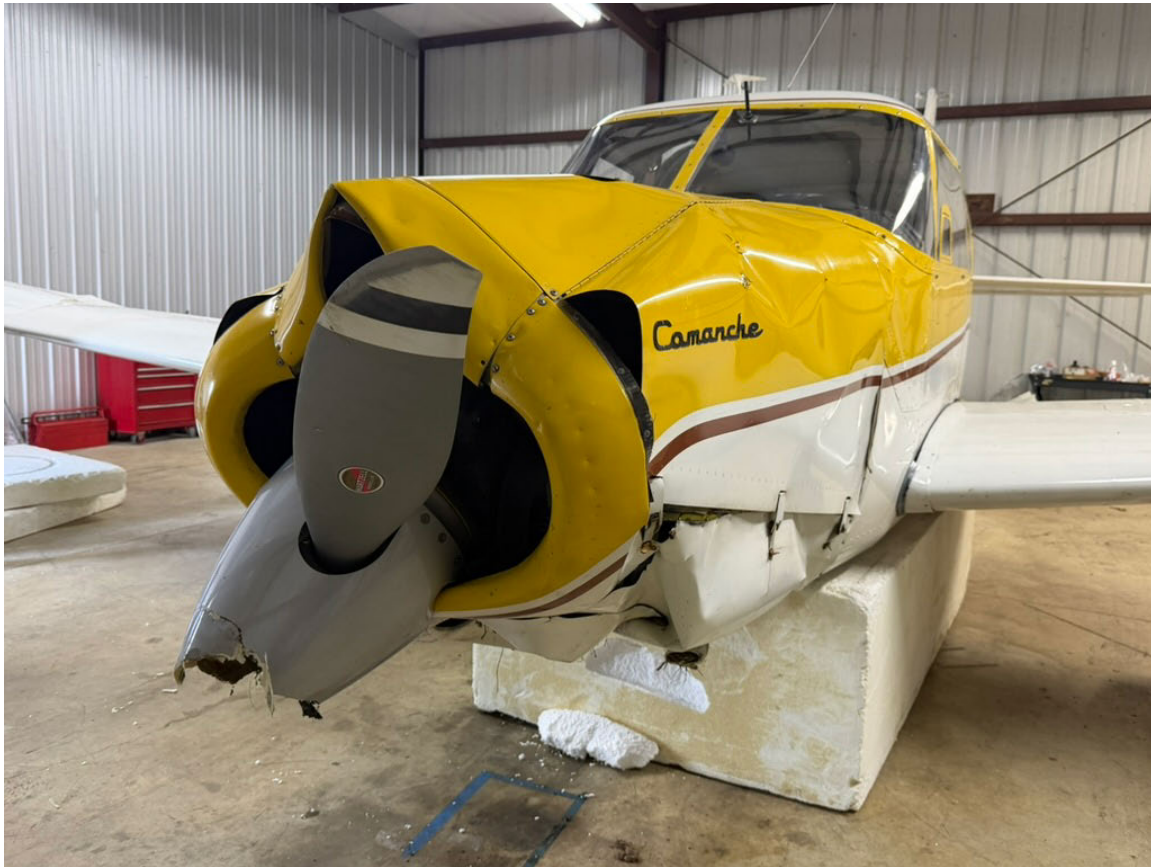
Figure 5: Forward fuselage and nose section of the aircraft showing impact-related deformation and damage.
