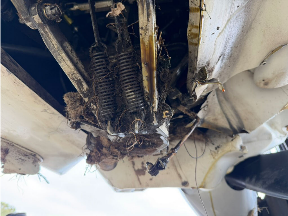
Figure 2: Nose landing gear assembly showing separation and structural damage at the nose gear attachment area.
