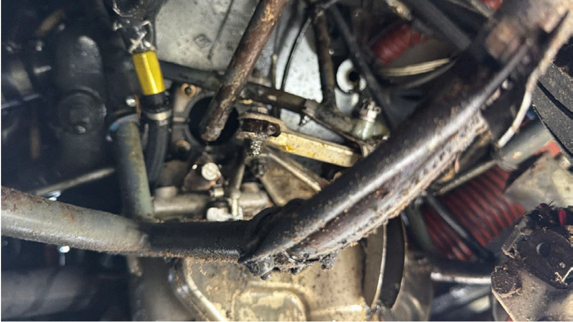
Figure 1: Nose landing gear steering linkage showing sheared pushrods at steering collar interface.
