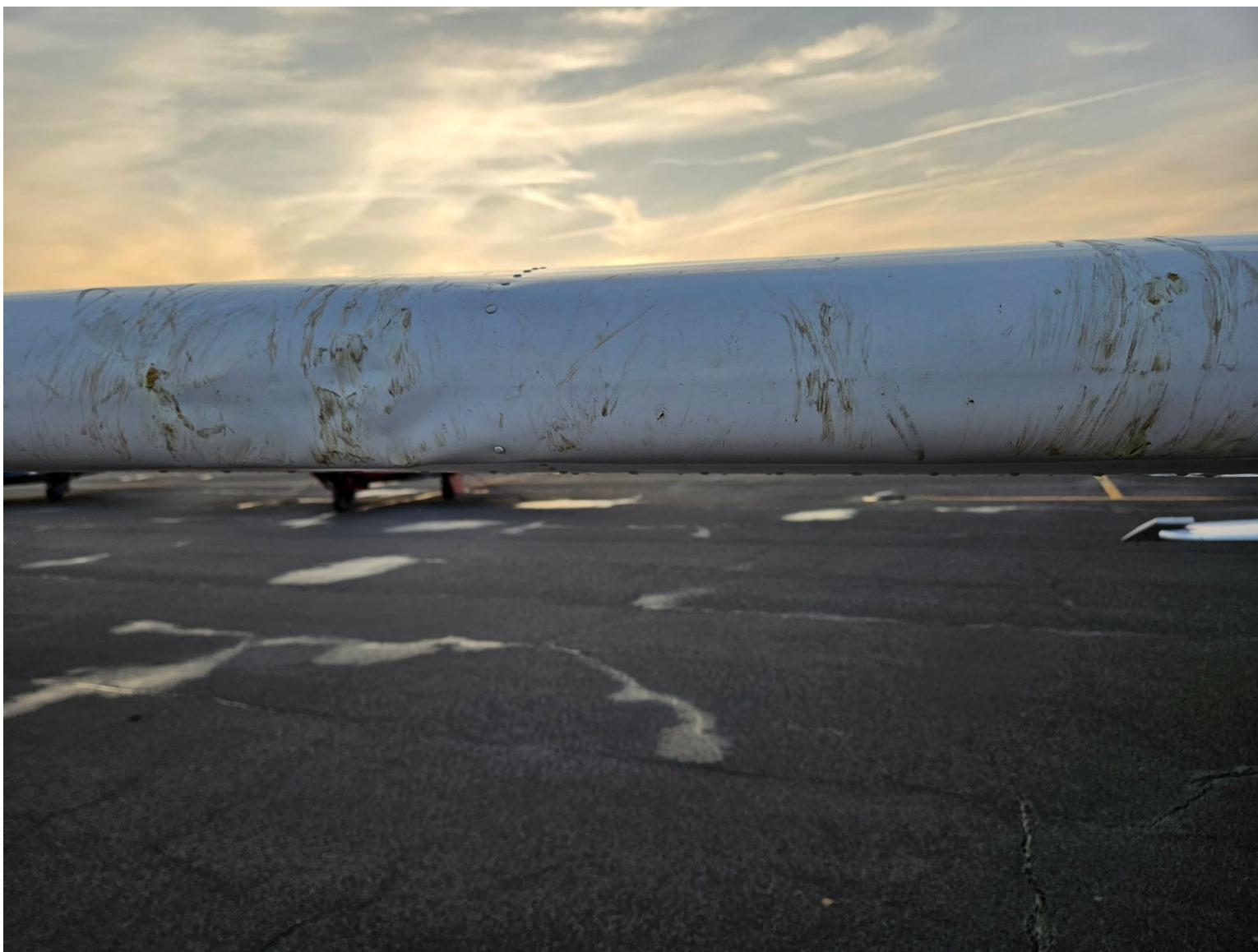
Photograph 3 - Damage to the right wing (Source: Wings of Carolina)
