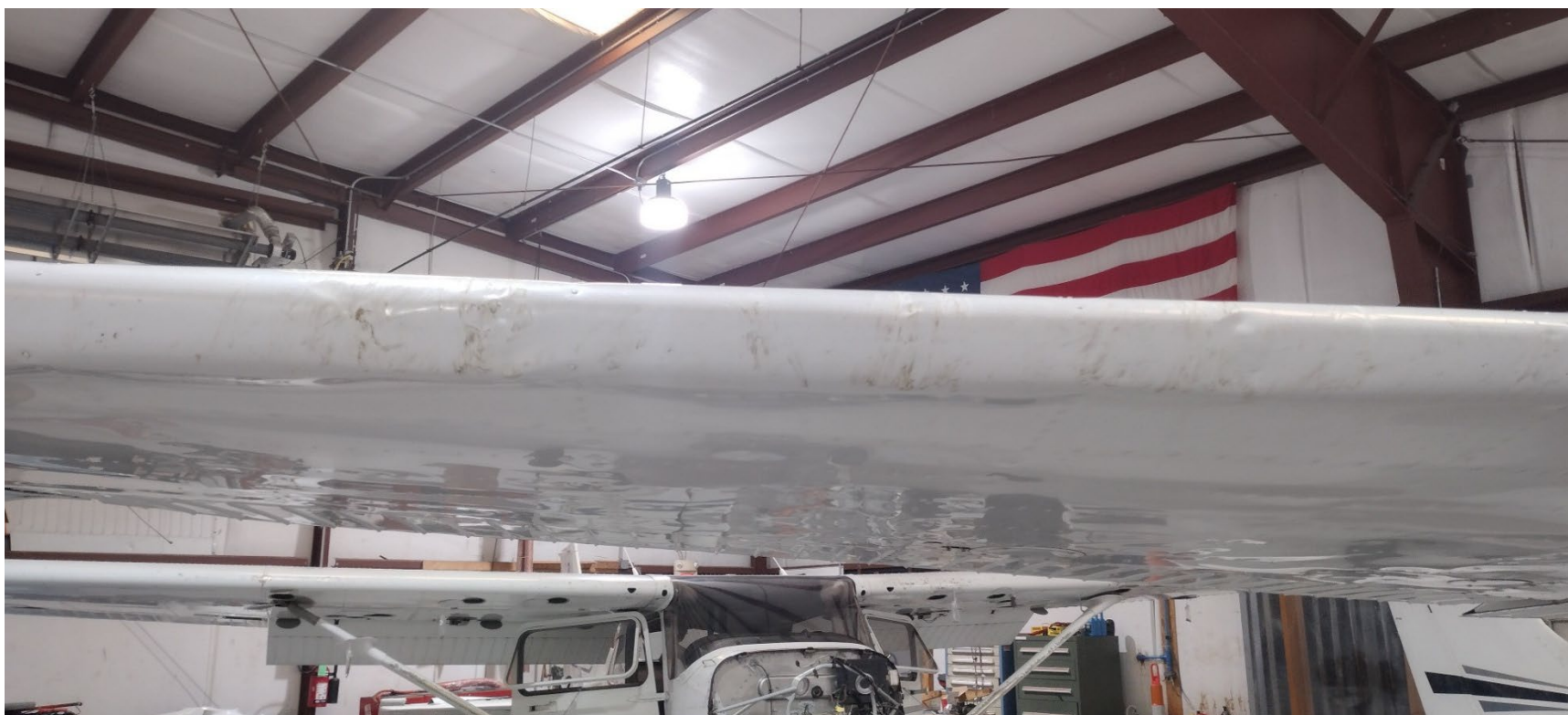
Photograph 5 - Damage to the right wing (Source: Wings of Carolina)
