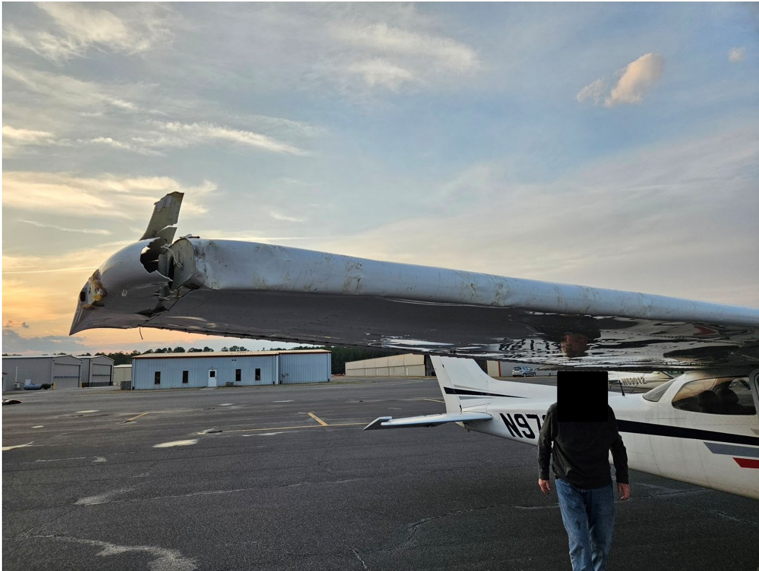
Photograph 1 - Damage to the right wing (Source: Wings of Carolina)
