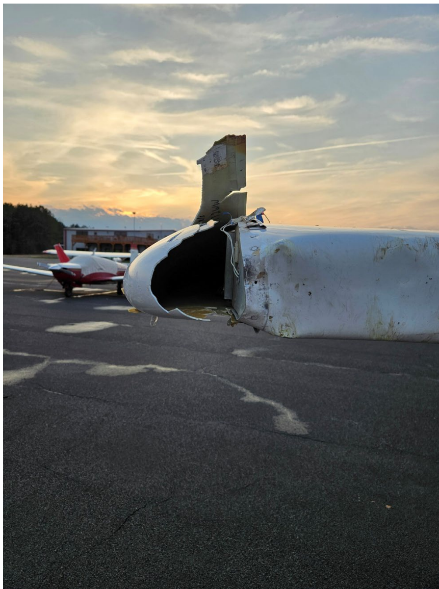
Photograph 2 - Damage to the right wing (Source: Wings of Carolina)
