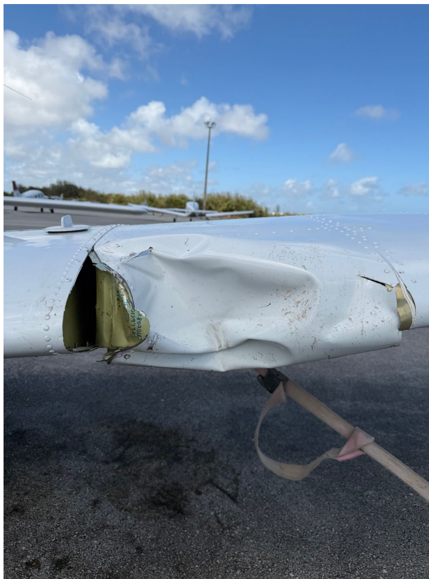
Photograph 2 - Bird strike damage to left leading edge. (Courtesy of Operator)
