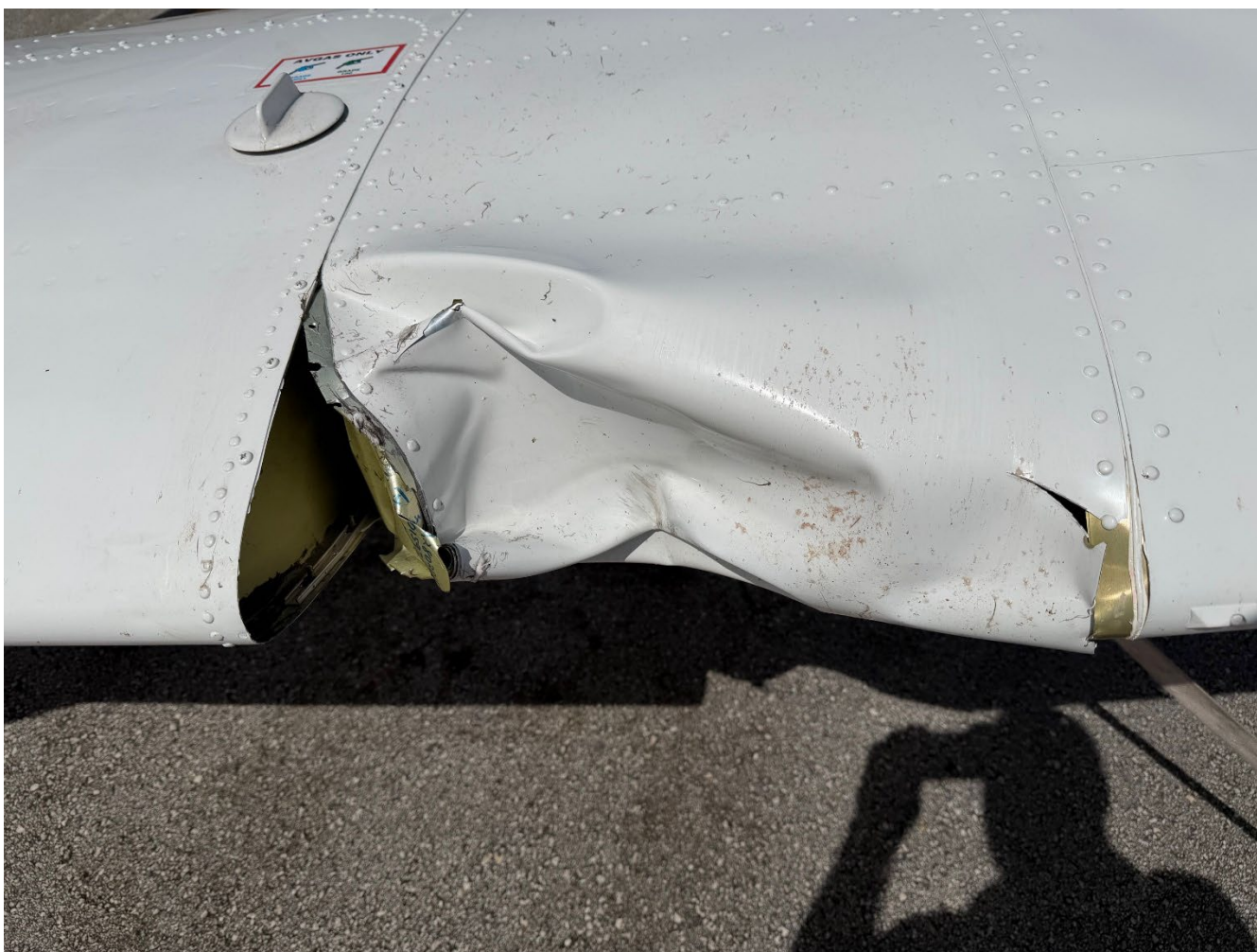
Photograph 1 - View of left wing damage caused by bird strike. (Courtesy of Operator)
