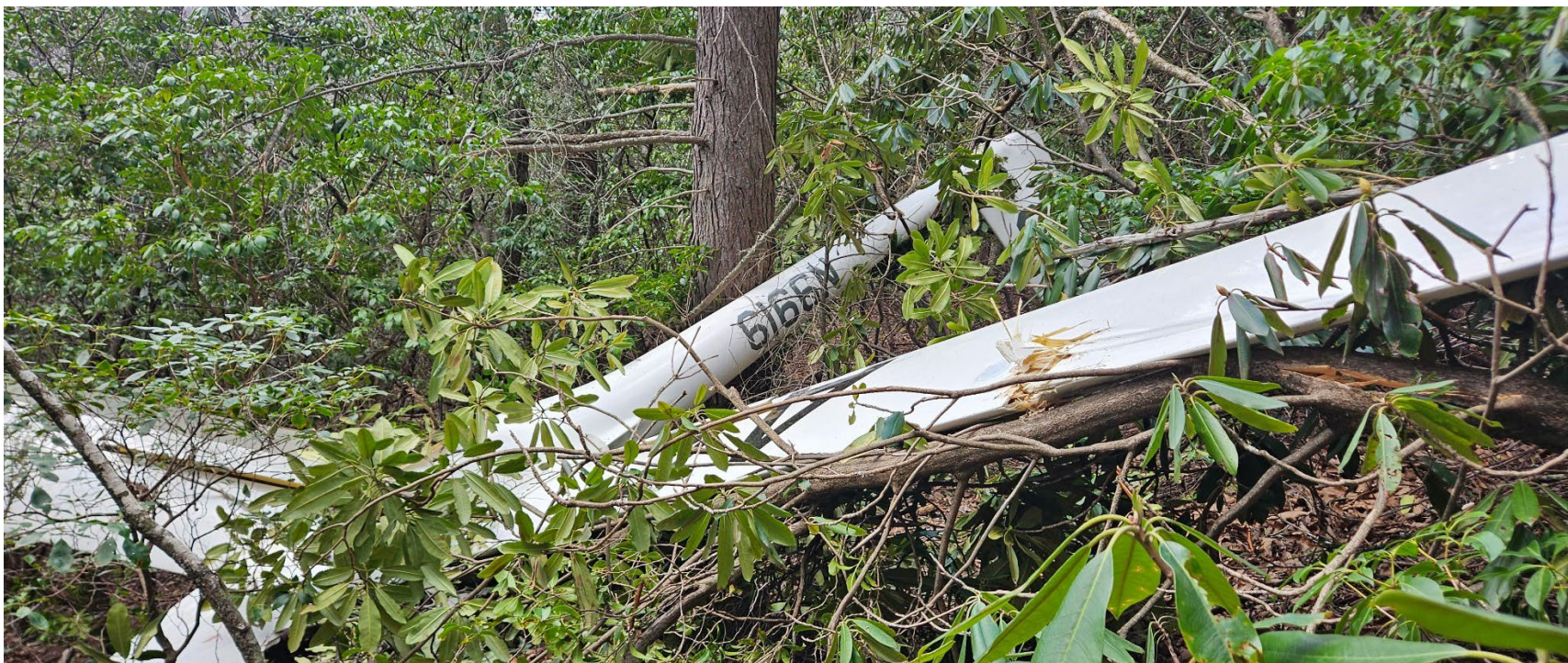
Photograph 1 - Right Forward Quartering View of the Inverted Glider at the Accident Site. Note the Partial Chordwise Fracture of the Right Wing (Courtesy of FAA)
