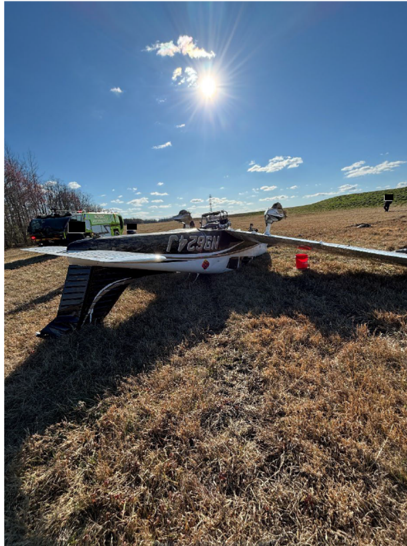
Photograph 3 - Aft view of airplane with damage to vertical stabilizer and rudder. (Courtesy of FAA)
