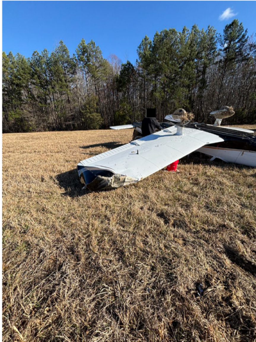
Photograph 4 - Left wing and tip damage. (Courtesy of FAA)
