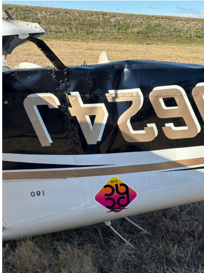
Photograph 2 - Right side fuselage damage. (Courtesy of FAA)
