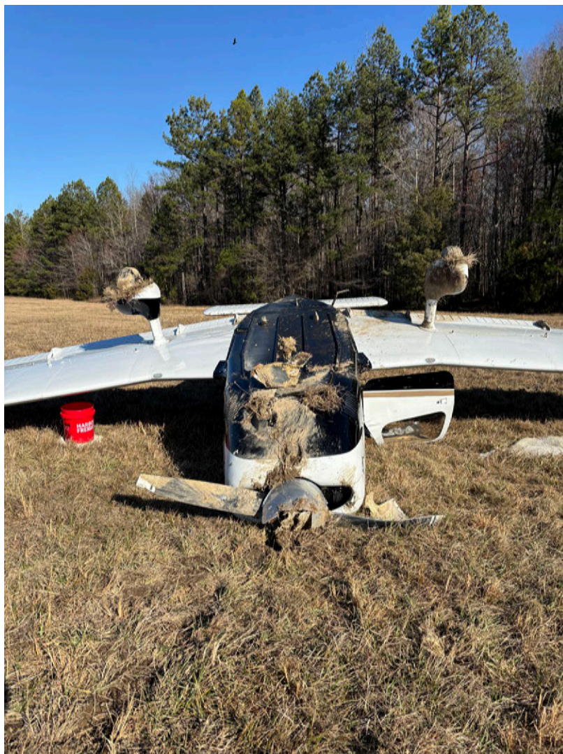
Photograph 1 - Airplane postaccident with fuselage damage at the step and across to the other side of the belly. (Courtesy of FAA)
