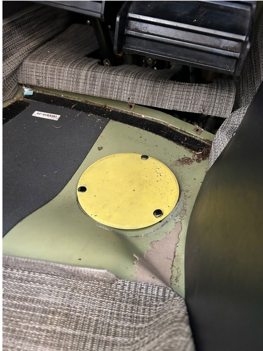
Photograph 5 - Close-Up View Showing Buckling Damage to Pilot's Side Floor (Courtesy of Operator)
