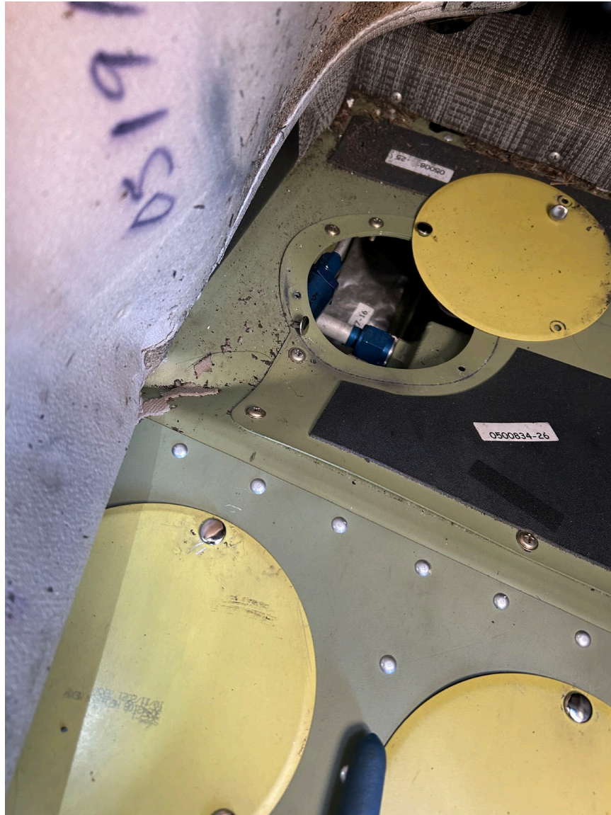
Photograph 6 - Close-Up View Showing Buckling Damage to Co-Pilot's Side Floor (Courtesy of Operator)
