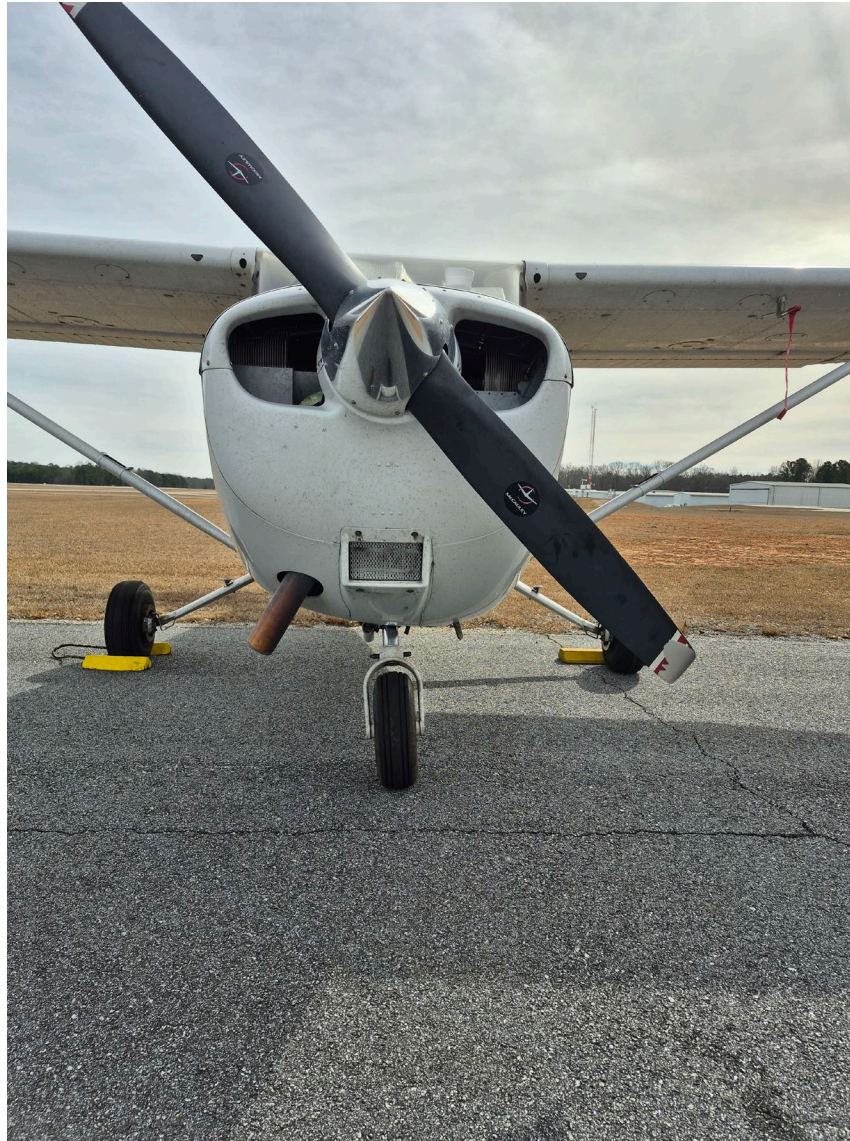
Photograph 1 - Frontal View of the Airplane on the Ramp Note the damaged lower Propeller Blade (Courtesy of FAA)
