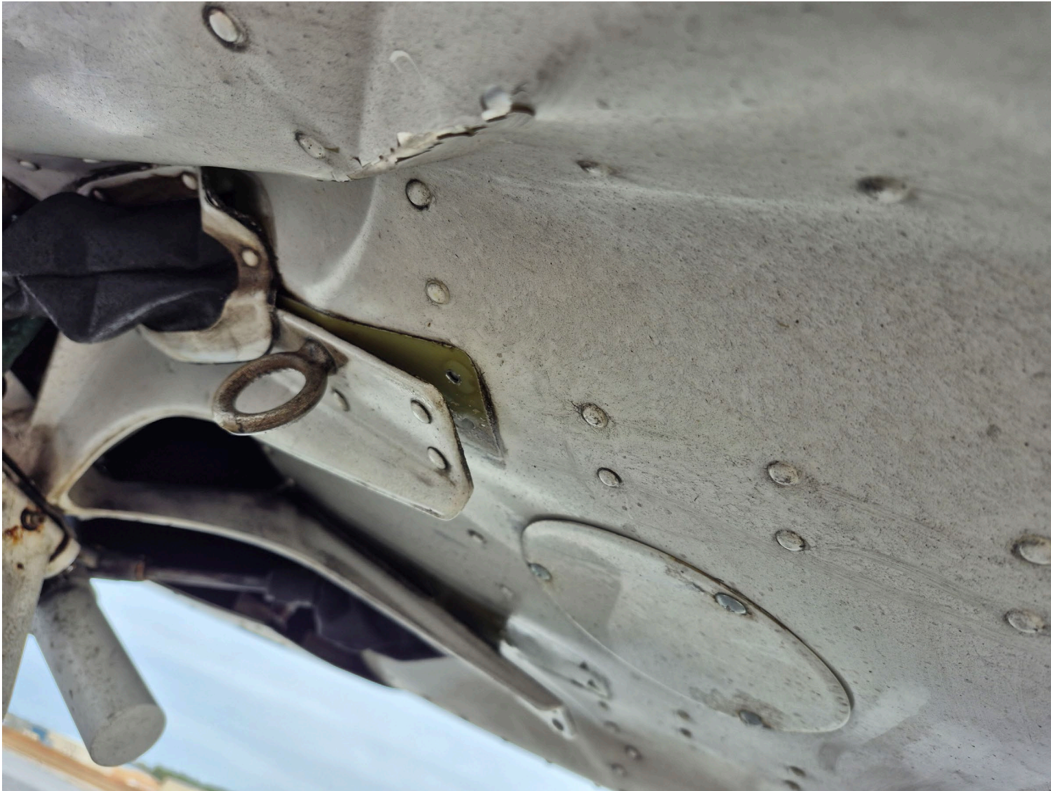
Photograph 3 - View of the Bottom Fuselage Showing Structural Buckling Damage Adjacent to Lower Nose Gear Fitting, Near Fuselage Station 0 (Courtesy of FAA)
