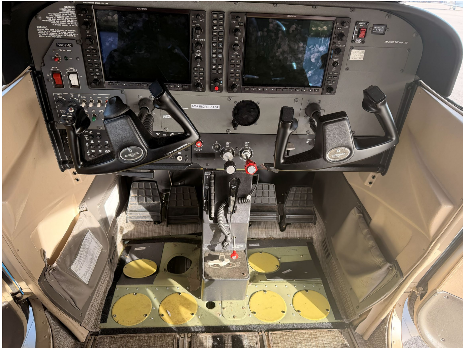
Photograph 4 - View of the Cockpit Showing Buckling of Floor on Pilot and Co-Pilot Locations (Courtesy of Operator)
