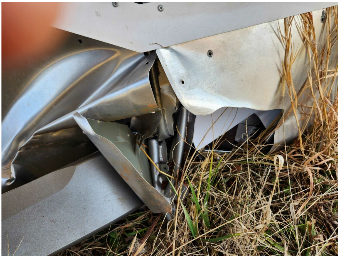
Photograph 4 - Broken frame on left side of fuselage (Courtesy of Owner)
