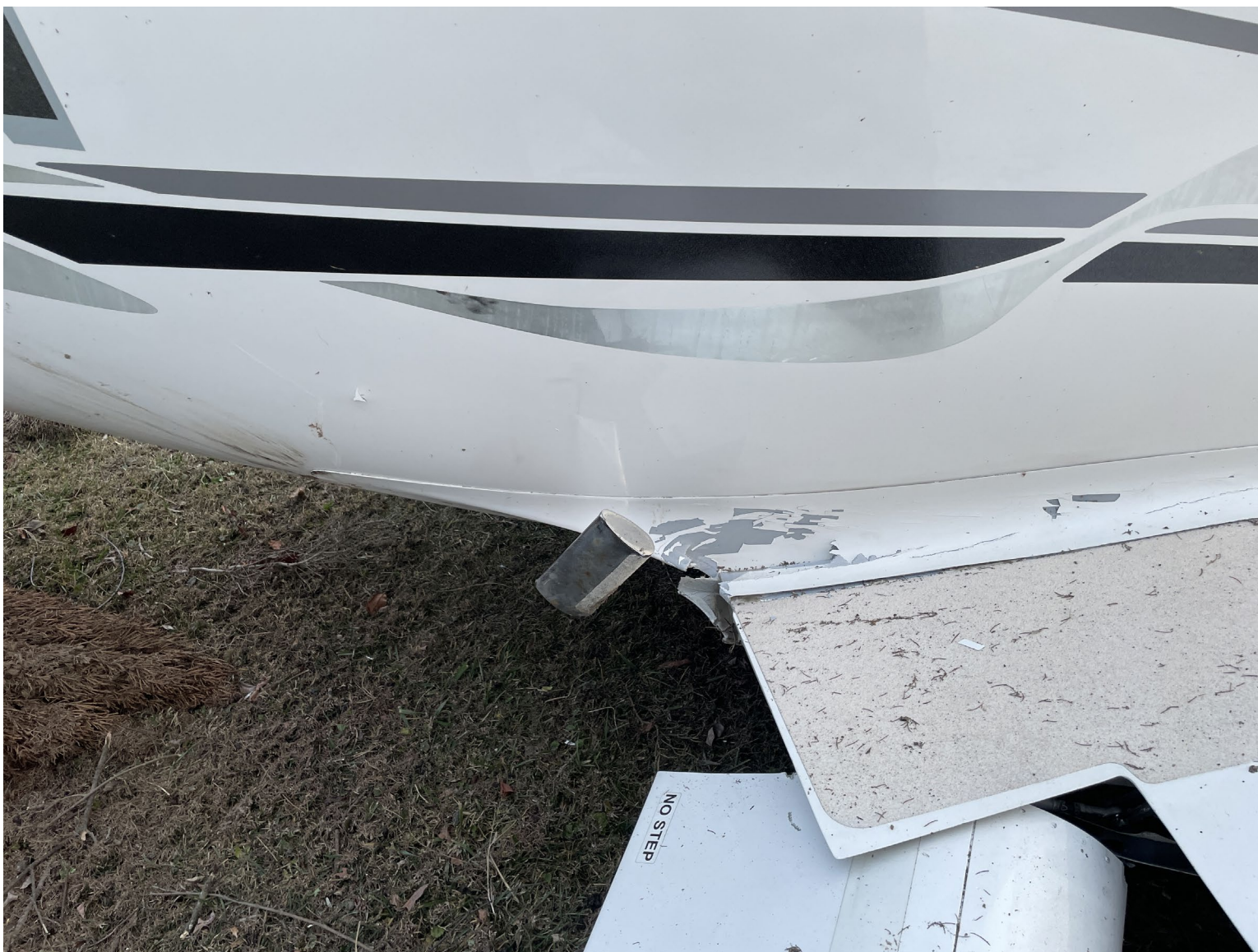
Photograph 3 - View of damage to the right wing root. (Courtesy of FAA)
