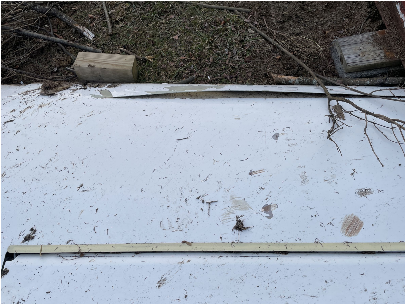
Photograph 2 - View of damage to the right wing leading edge. (Courtesy of FAA)
