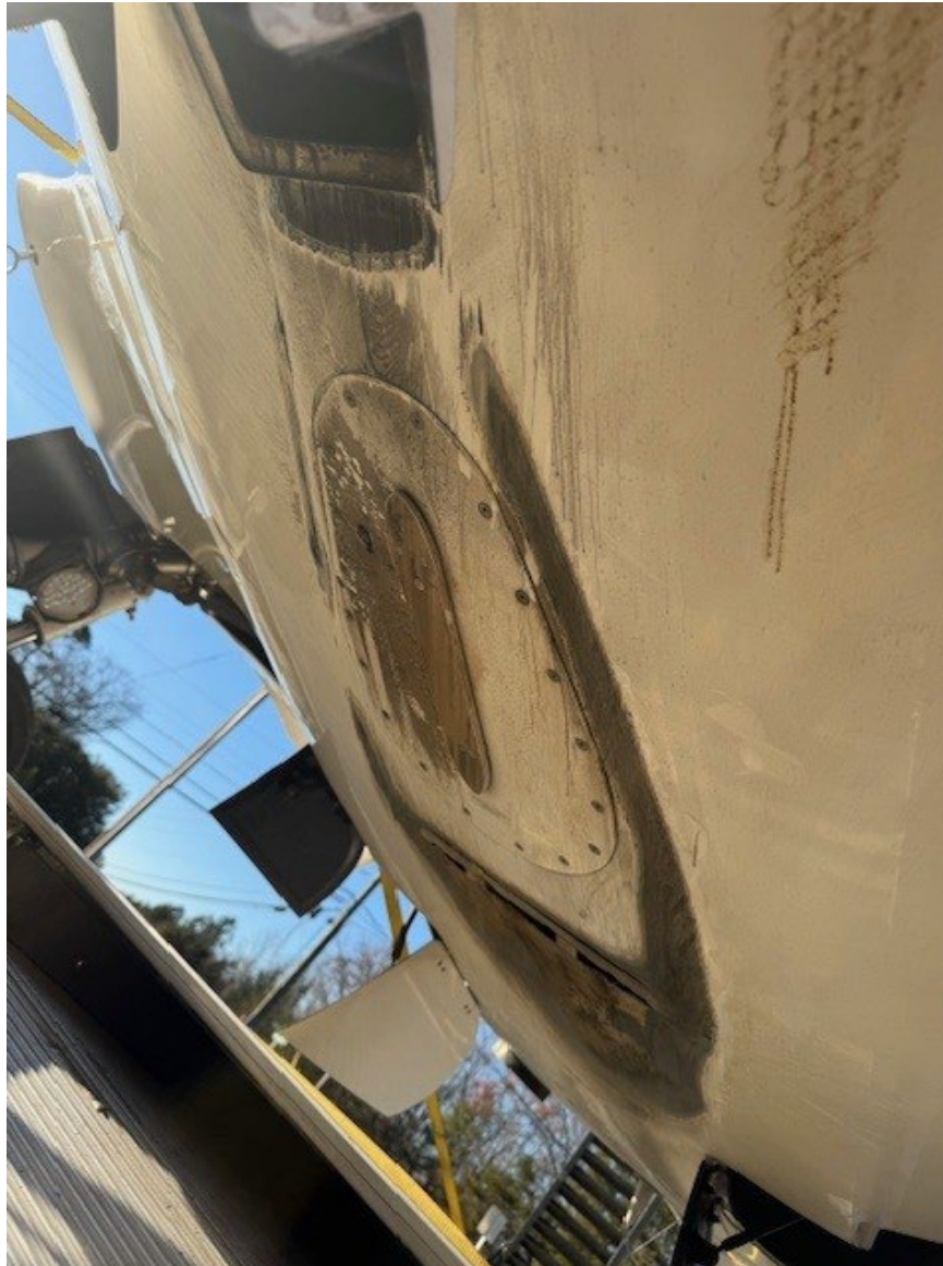
Photograph 3 - Damage to Lower Fuselage (Courtesy of FAA)
