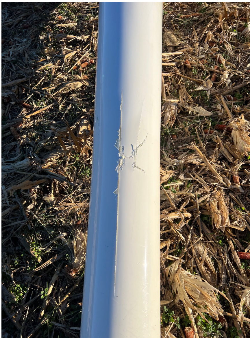
Photograph 2 - Fuselage Damage (Courtesy of FAA)
