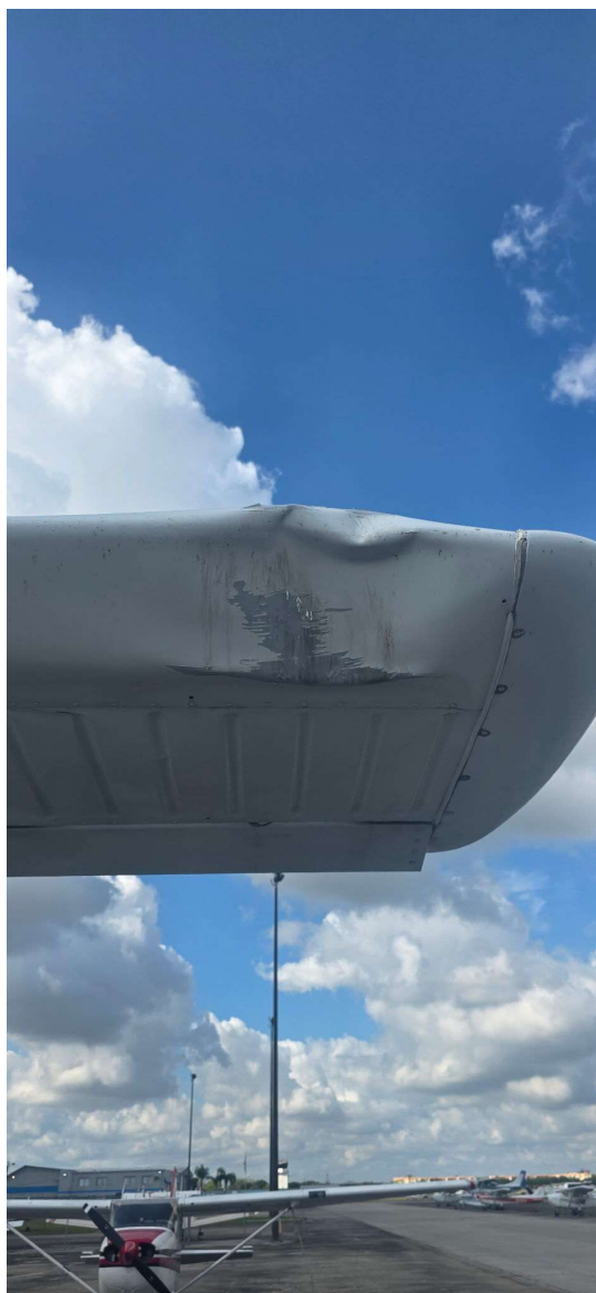
Photograph 2 - Close up of damage to left side of horizontal stabilator (Courtesy of Pilot)
