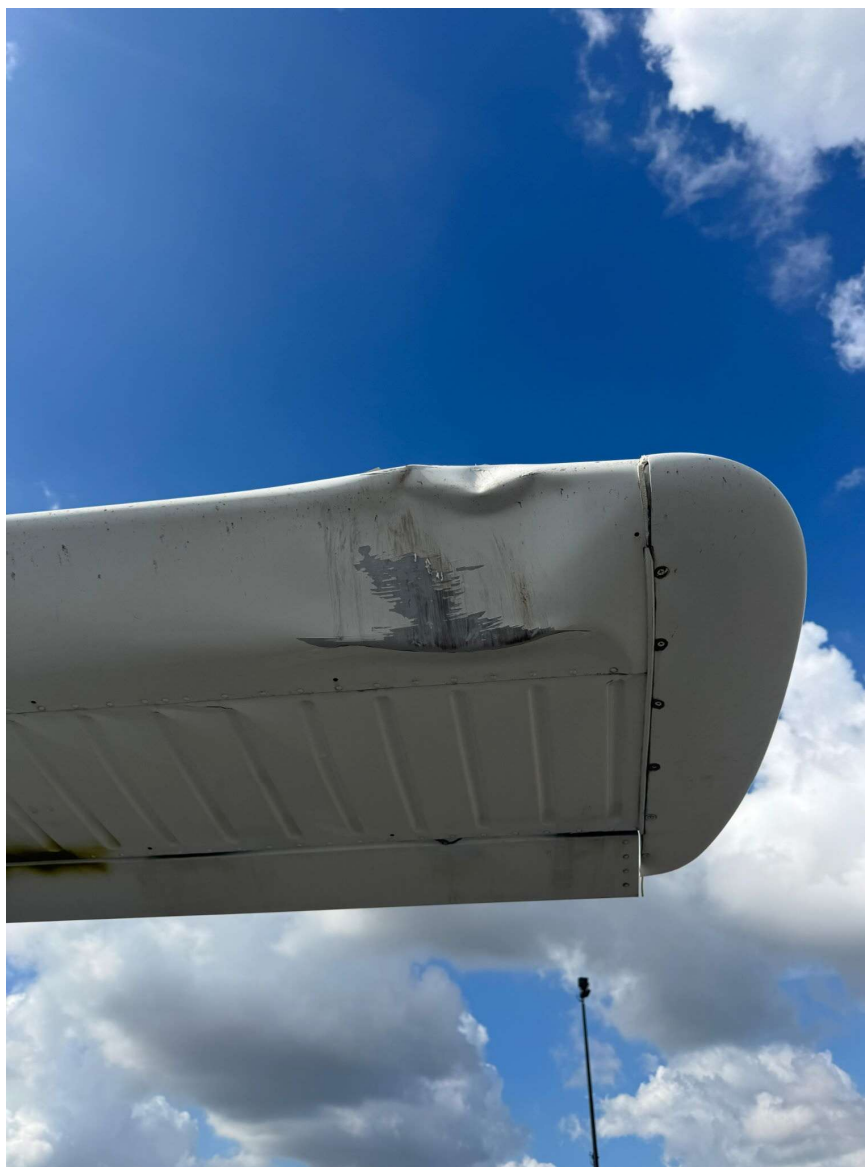
Photograph 3 - Close up of damage to left side of horizontal stabilator (Courtesy of Pilot)
