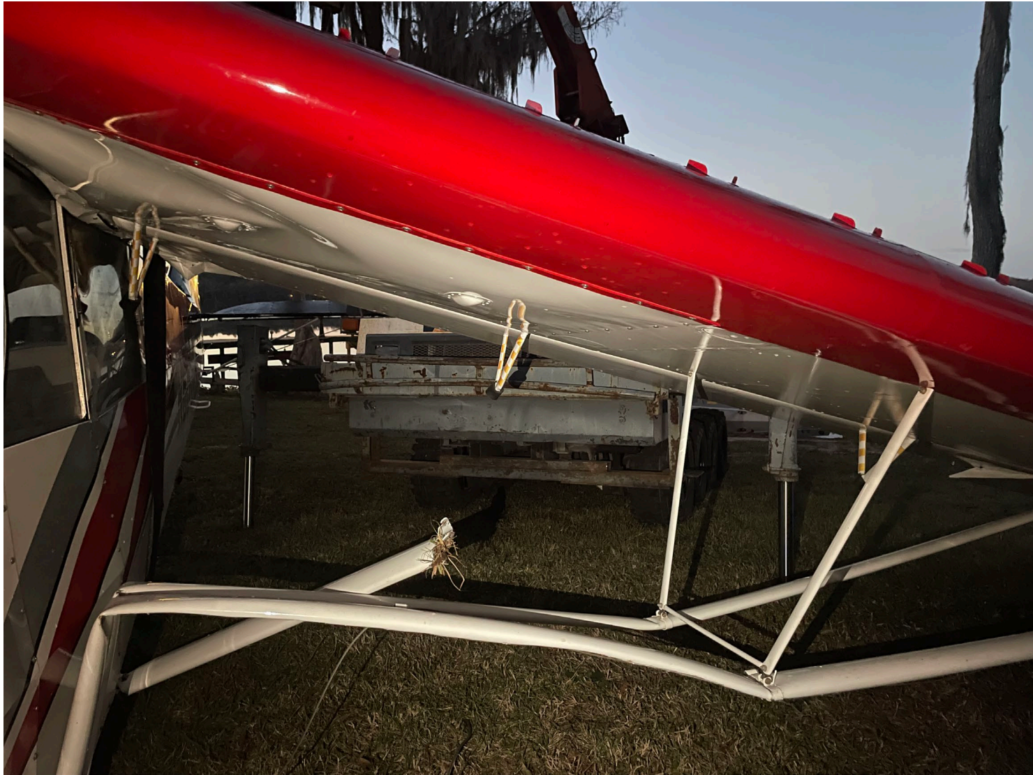
Photograph 3 - Left Wing Strut Buckled (Courtesy of FAA)
