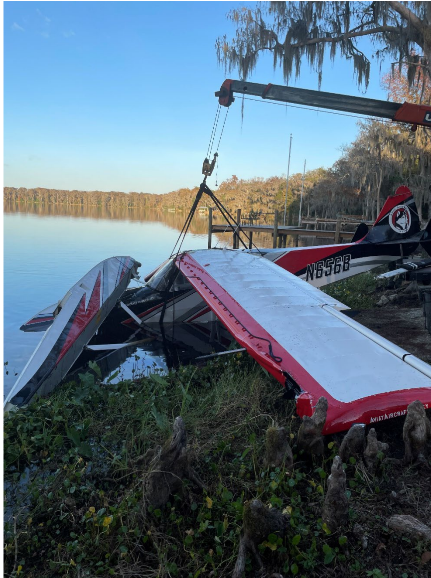
Photograph 2 - Left-Wing Leading Edge Damage Shown During Recovery (Courtesy of FAA)
