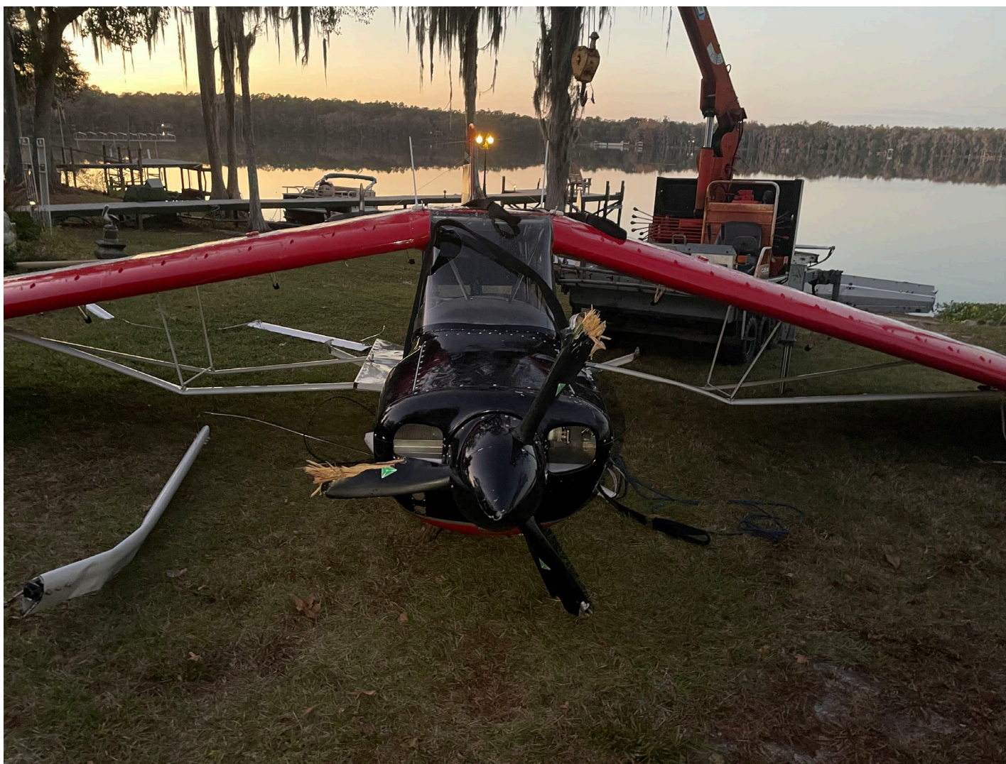
Photograph 4 - Propeller, Fuselage, Windshield and Wing Strut Damage (Courtesy of FAA)
